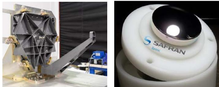
**Fig. 5.** Telescope (designed by Airbus Defence and Space) and secondary mirror (SAFRAN)
