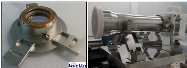
**Fig. 6.** Entrance Filtering Optics and Blocking Filter (FM models) produced by Bertin Technologies
