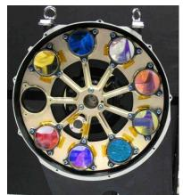
Fig. 1. Example of a set of optical interference filters fixed on a filter wheel and dedicated to the GOCI instrument installed on the COMS satellite [1]
