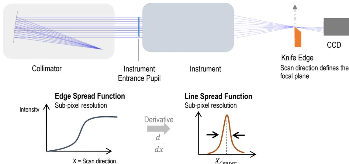
**Fig. 4.** Principle of the knife-edge test used for instrument spatial resolution measurement
