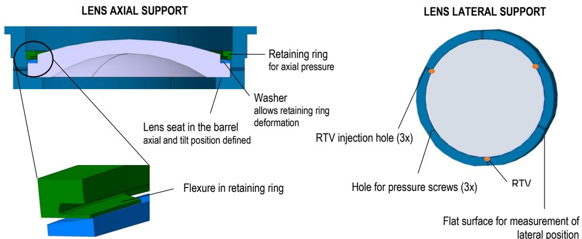
Fig. 1. Lens axial and lateral support
