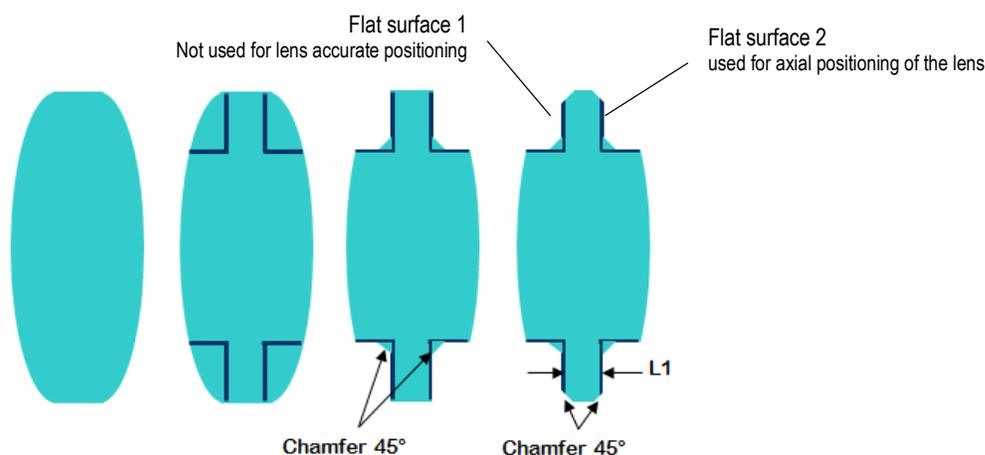
**Fig. 2.** Flat machining of FIMAS lenses
