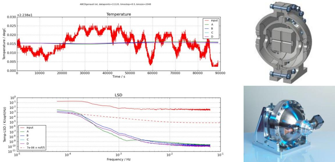
**Fig. 5** Top left: GOCE Temperature time series (input) and temperature time series of the cavity for different coating variants. Bottom left: The corresponding linear spectral densities (A - no gold coating, no multi layer insulation(MLI); B - no gold coating, MLI; C - all surfaces gold coated, MLI; D - all surfaces but cavity gold coated, MLI). Right: schematic cross section through the cavity and a picture of the constructed EBB LSU
