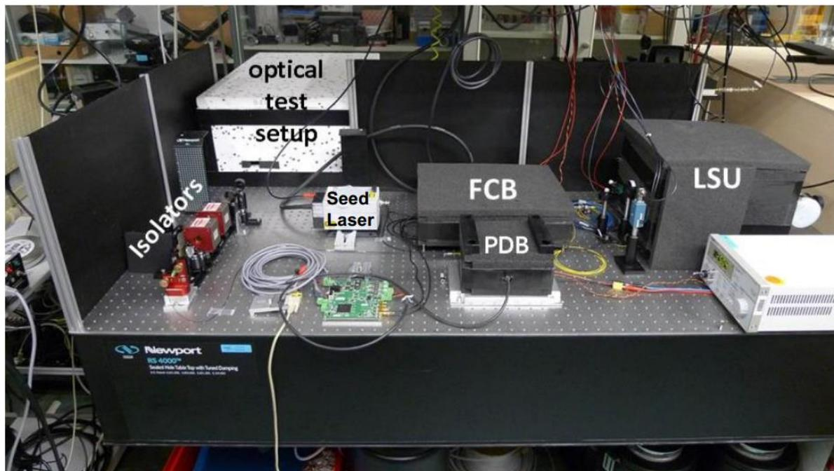
Fig. 8 HSL EBB test configuration in Airbus D&S lab
