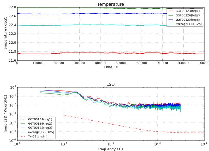
**Fig. 2** GOCE thermal noise environment of regulated platform, measured time series and linear spectral density
