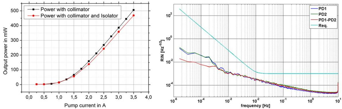
Fig. 6 Left: LH output power; right: LH Output power stability
