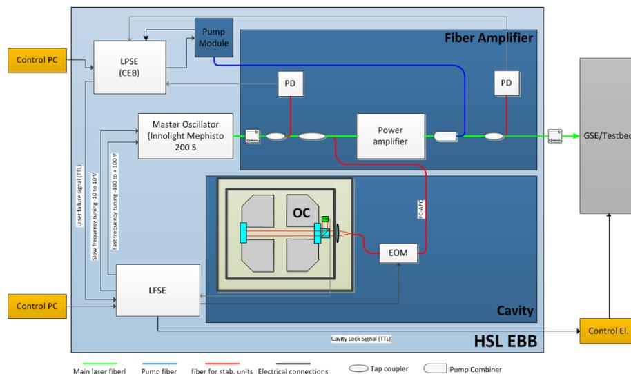
**Fig. 1** HSL setup (LPSE=laser power stabilisation electronics; LFSE=laser frequency stabilisation electronics)
