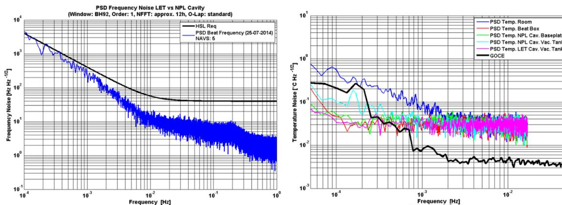
Fig. 9 Left: Frequency stability measurement(master oscillator and cavity only) ; right: temperature environment in the lab, compared to the GOCE thermal environment
