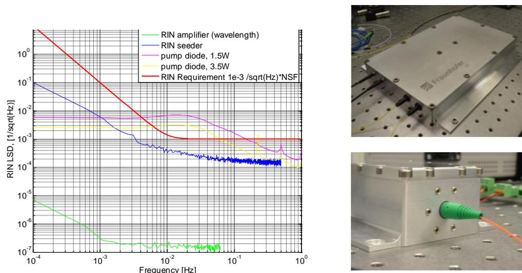
**Fig. 4** Left: RIN of the Laser head due to different sources; right: LH EBB boxes
