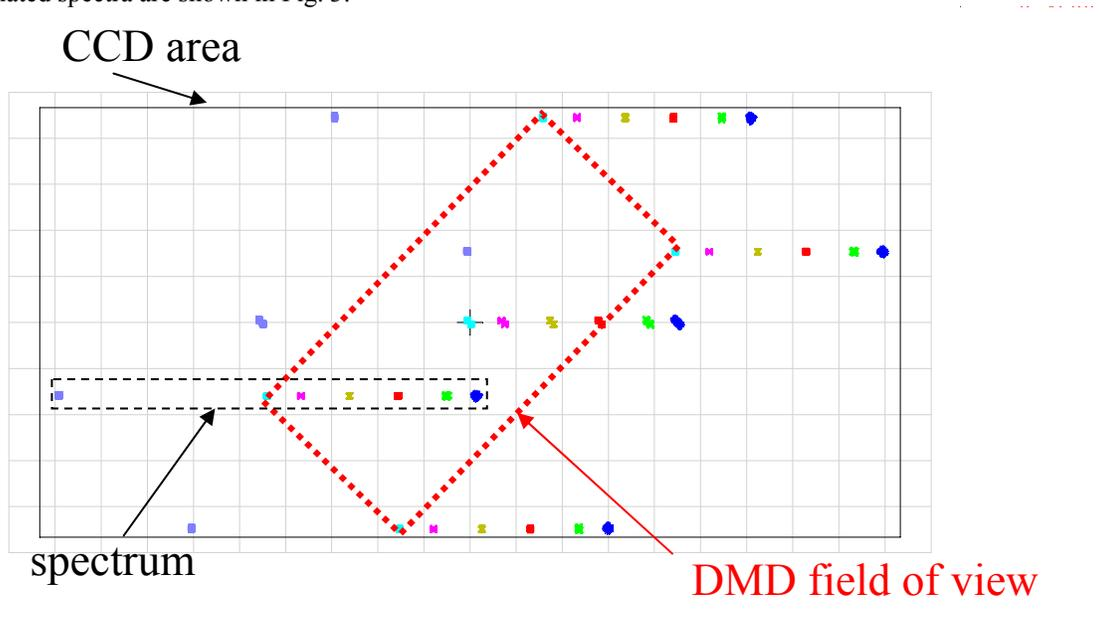
**Fig. 3.** Spectroscopic channel; simulated spectra on the detector.
