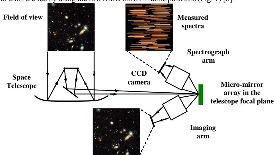
Fig. 1. Principle of BATMAN spectro-imager
