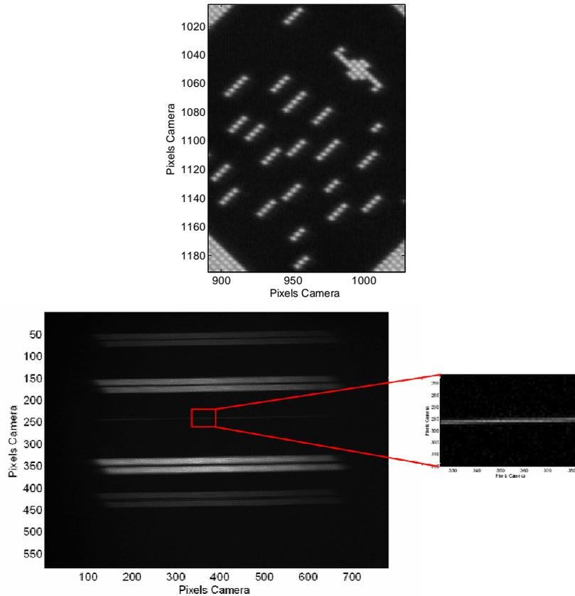
**Fig. 6.** (a) Image of a typical slit mask in the imaging channel; (b) spectra in the spectral channel, including a single micromirror slit (close view of the spectrum generated by the one-micromirror slit)
