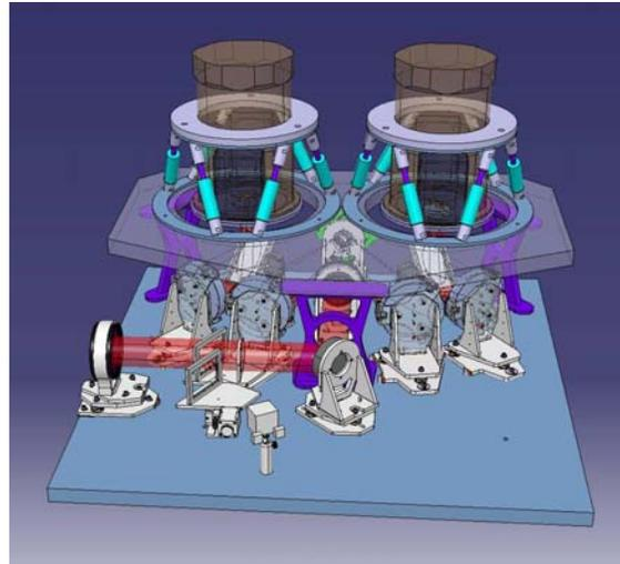
**Fig. 4.** BATMAN opto-mechanical design.
