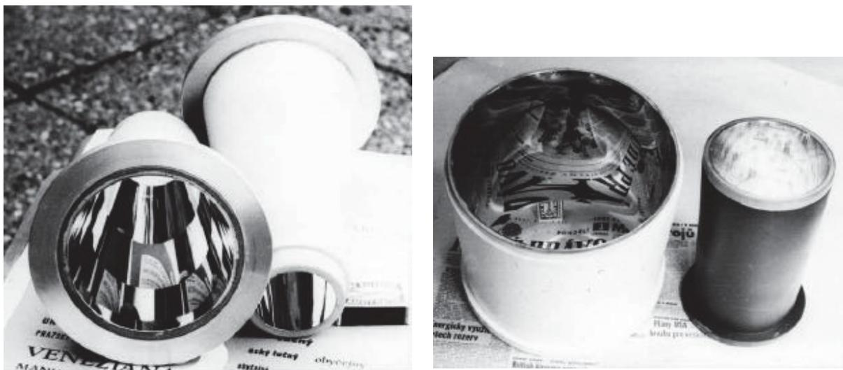
Fig. 2: Mirror shells of the Salyut 7 X-ray mirror assembly, 1981
