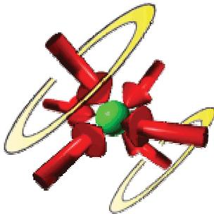
Fig. 2. Scheme of a magneto-optical trap : a cloud of about  $10^9$  atoms (in green) is cold and trapped. The laser beams (in red) exert a viscous force on the atoms whose velocity decrease from  $100 \text{ m.s}^{-1}$  to a few  $\text{mm.s}^{-1}$ . The width of the atomic velocity distribution is decrease in the same way. The magnetic gradient
