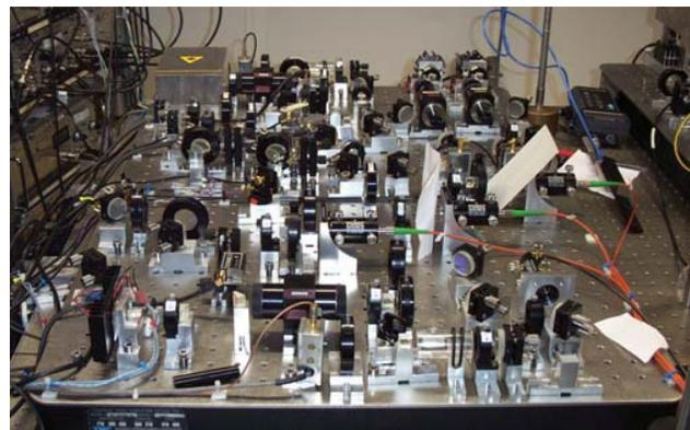
Fig. 1. Photography of a laser cooling bench used at the BNM-SYRTE (Paris Observatory) for an experiment
