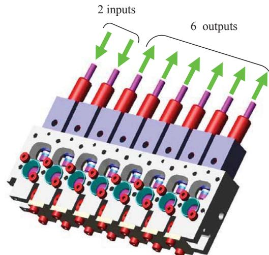
Fig. 5. Design of a splitter with 2 inputs and 6 outputs using miniature optical components (half waveplates and polarizing beam splitters).
