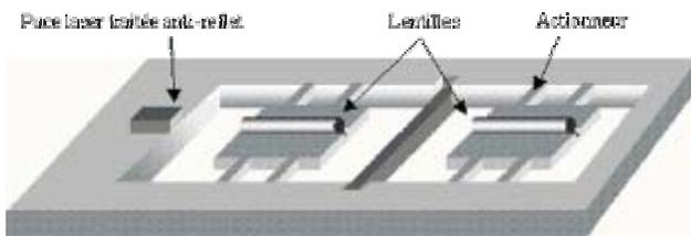
Fig. 4. Scheme of the ECL developed at the LPMO. The cavity is made by two selfoc lenses fixed on MEMs thermal actuators to control and stabilize the emitted wavelength.
