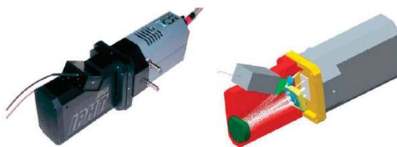
Fig. 4. MIRAS II spectrometer with commercial CCD detector (left) and schematic view of the folded optical path (right).
