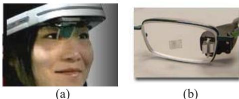
Fig.3. Example of commercial HMD. (a) Nomad from Microvision. (b) EG-8 from MicroOptical.
