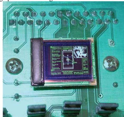
Fig.6. Photography of the SVGA+ OLED microdisplay.
