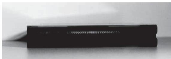
Fig. 7 . The Angel LE linear prototype (47 cells 2.5 x 25.5 mm, 120 mm long).
