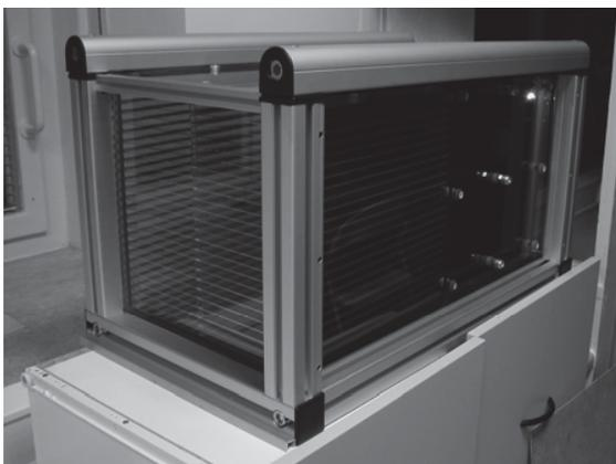
Fig. 4. The large (30 x 30 x 60 cm) LE 2 D module (0.75 mm thick gold coated glass plates). The array can be re-designed and re-shaped to achieve the approximation of a K-B, or alternatively, of a XEUS (i.e. Wolter) geometry, these modules have been also designed and developed.
