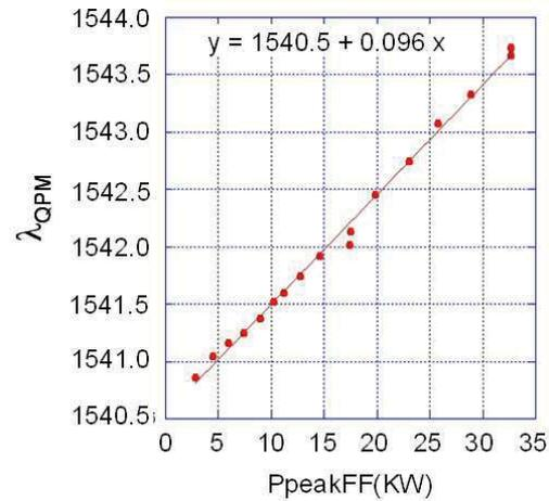
Fig. 5. Measured SH peak drift vs FF power.
