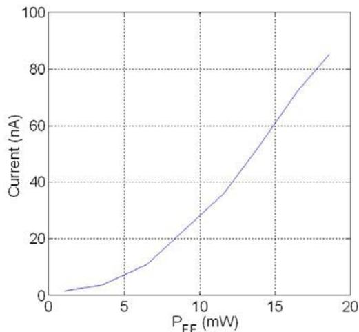
Fig. 7. Quadratic behaviour of generated UV light (photodiode current) versus pump power.
