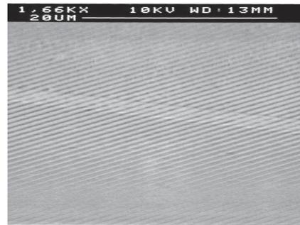
Fig. 2. Poling on a  $\alpha$ -phase PE waveguide.
