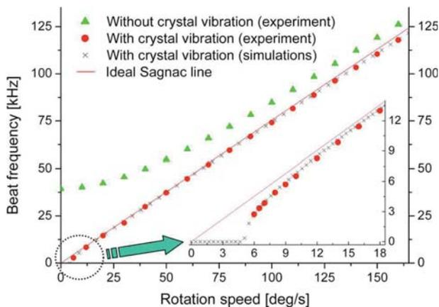
Figure 2 : Experimental frequency response curve of our prototype solid-state ring laser gyro with (circle marks) and without (triangle marks) crystal vibration. Also shown (crosses) is the result of numerical simulations in the vibrating crystal case.
