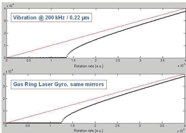
Figure 3 : Comparison of the frequency responses of the solid-state ring laser gyro with vibrating crystal (above) and of the Helium-Neon ring laser gyro (below) with identical values of the mirror-induced backscattering coefficient (numerical simulations).
