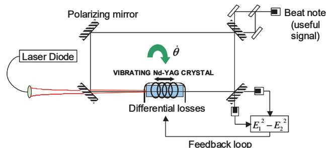
Figure 1 : Basic experimental setup of a solid-state ring laser gyro
