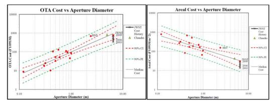
Fig 3: OTA Cost vs Aperture Diameter scaling law for 17 free flying UV/OIR systems (including 2009 JWST). Plot includes 90% confidence and prediction intervals, and data points. Chandra data is not in the regression.
