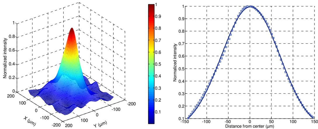
**Fig.4.** At the predicted best position: on the left, PSF; on the right, cross section (square are measured points, line is a Gaussian fit)
