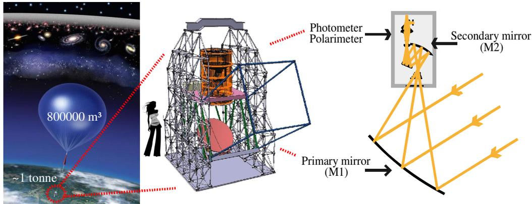
Fig.1. From left to right, a representation of the stratospheric balloon and onboard experiment, the instrument in the pointed payload, the optical concept
