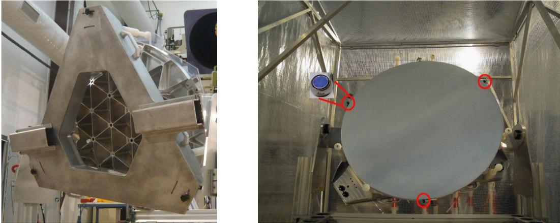
**Fig.2.** Primary mirror on his test support: on the left, view on the lightened part; on the right, view on the optical part, red circle indicates the position of the three reflectors balls
