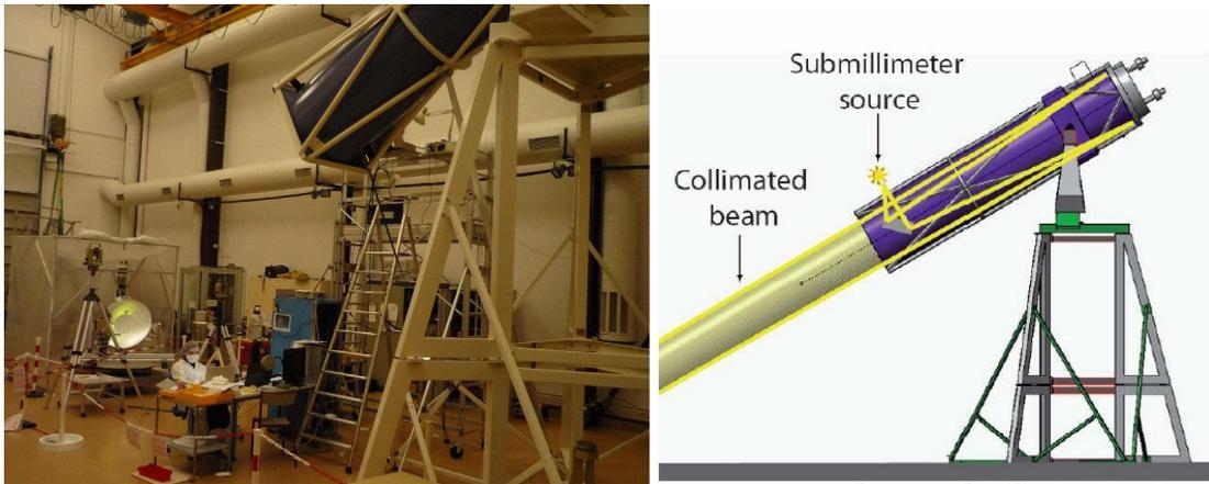
**Fig.3.** On the left, primary mirror under characterization; on the right, representation of the 1m diameter collimator and the incident submillimeter collimated beam (at an elevation angle of 30°)
