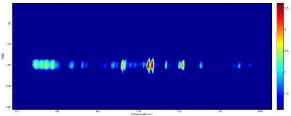
Fig. 1. EUV detector Image for Argon gas: HV = -3436 V, this image corresponds to a cumulated integration time of 10 min. The count rate is about 1500 counts per second. (Levels are in  $log_{10}$ -scale)
