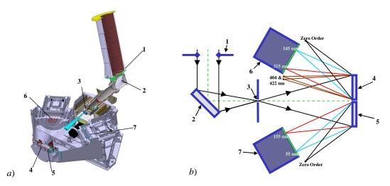
**Fig. 1**. *a*: PHEBUS instrument, *b*: Optical configuration 1 – Entrance pupil; 2 – Entrance mirror; 3 – Slit; 4 – FUV grating; 5 – EUV grating; 6 – FUV detector; 7 – EUV detector
