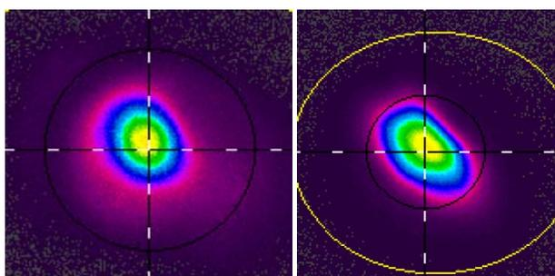
**Fig. 4.** Beam profiles of the MOMA laser head. Left: configuration with short nonlinear crystals, rather circular beam profile. Right: configuration with long nonlinear crystals, rather elliptical beam profile due to walk-off in the crystals.
