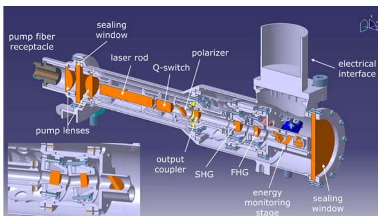
**Fig. 2.** Mechanical design of the MOMA laser head
