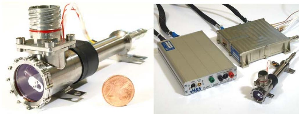
**Fig. 3.** Right: MOMA laser head. Left: MOMA laser system consisting of laser head (front right), pump unit (back right, by vH&S), GSE interface (left, by vH&S)
