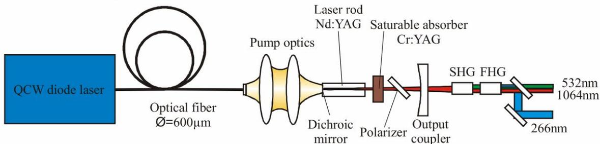
Fig. 1. Optical concept of the laser
