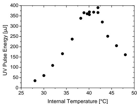
**Fig. 5.** UV pulse energy in dependence on the internal operating temperature (which is the temperature of the frequency conversion crystals).
