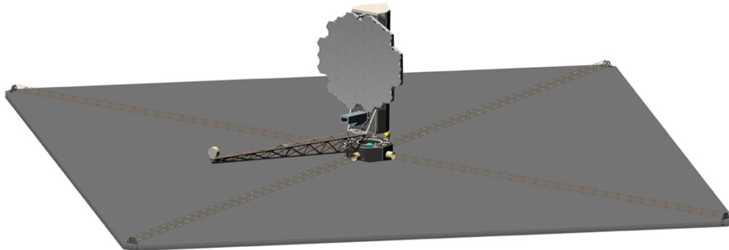
Figure 3: The LUVOIR-B observatory, with an 8-m diameter off-axis primary mirror and three instruments bays. Deployment and pointing animation at <https://asd.gsfc.nasa.gov/luvoir/design/>. Credit: A. Jones (NASA GSFC)
