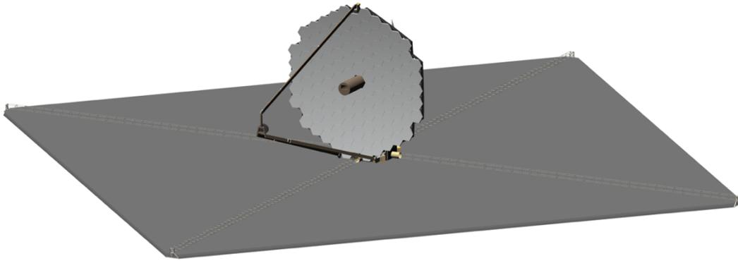
Figure 2: The LUVOIR-A observatory, with a 15-m diameter on-axis primary mirror and four instruments bays. Deployment and pointing animation at <https://asd.gsfc.nasa.gov/luvoir/design/>. Credit: A. Jones (NASA GSFC)
