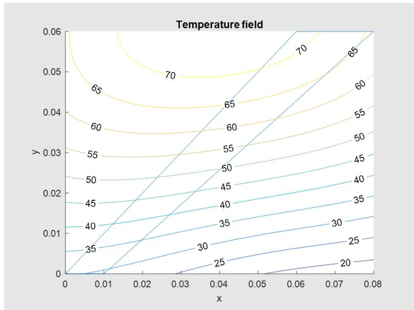
Figure 6. A 2D temperature field reconstruction results.
