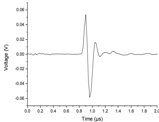
Figure 1. The ultrasonic signal generated by the fiber optic generator.
