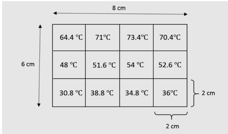
Figure 4. Reference temperature map recorded by the thermocouple.
