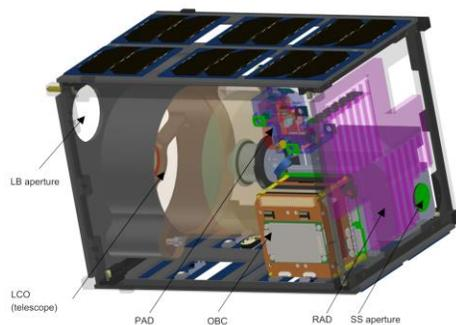
Figure 3. Schematic view of the main components of the light collection optics (LCO), polarization analysis and detection module (PAD), star tracker (SS), on-board computer (OBC), solar panels and the radiator (RAD) for passive detector cooling. Notably, the laser beacon (LB) with its telescope and the battery packs are not shown to provide an unobstructed view of the remainder.
