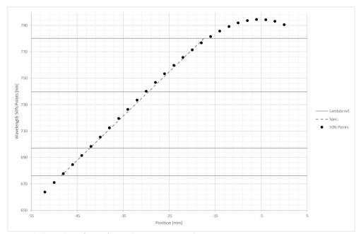
Figure 4. Measured 50% points of manufactured LVF versus requirements.
