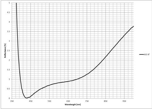
Figure 10. Measured reflectance of black coating at AOI 8°.
