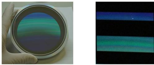
Figure 9. Pictures of manufactured LVF at wafer level (left) and with applied black mask (right).
