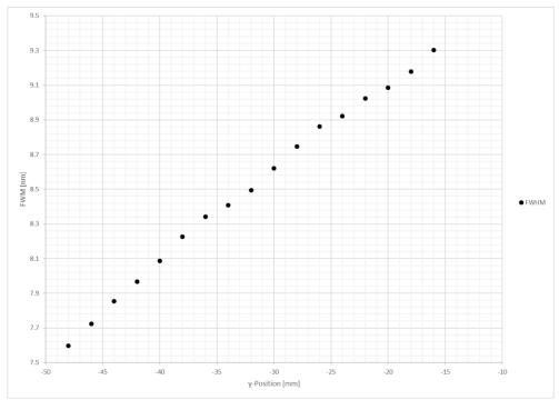
Figure 6. Measured FWHM along spectral direction.
