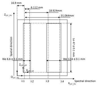
Figure 3. LVF design: HR1W and HRW2 dimensioning
