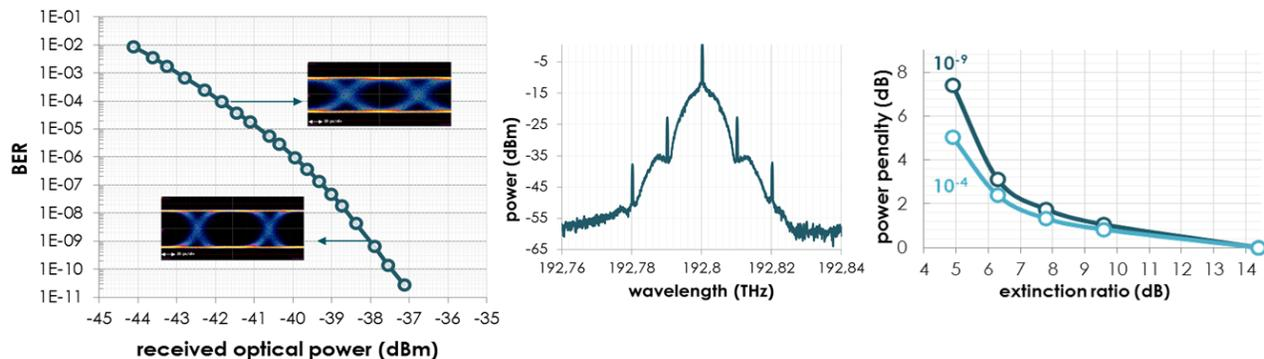
Figure 4. BER curve for a 10 Gbps NRZ OOK (left) with eye diagrams at  $10^{-4}$  and  $10^{-9}$  (inset), optical spectrum at Tx output (middle) and influence of the extinction ratio at  $10^{-4}$  and  $10^{-9}$ .
