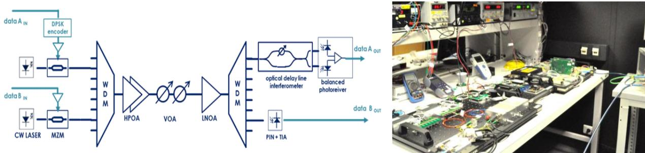
Figure 3. FSO communication link test-bed: (top) schematic with 2 OOK/DPSK channels, (bottom) picture of the set-up
