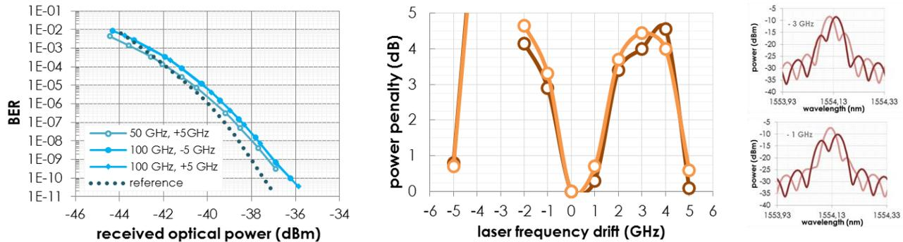
Figure 7. (left) BER at 10 Gbps OOK for wavelength drift of +/- 5 GHz for filters of 50 and 100 GHz bandwidth, (center) power penalty vs. wavelength drift for 10 Gbps DPSK, (right) output spectra (constructive and destructive ports) for -3 and -1 GHz offsets.
