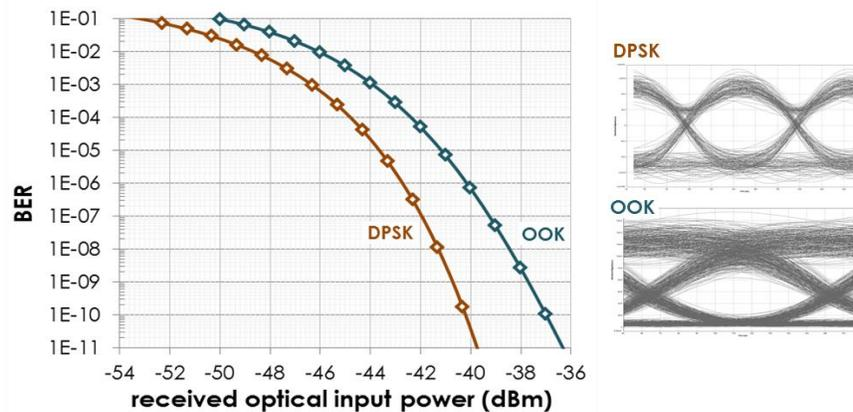
Figure 2. Simulated BER performance (left) and  $10^{-9}$  BER eye-diagrams (right) for 10 Gbps NRZ-OOK and NRZ-DPSK
