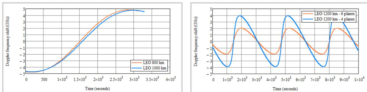
Figure 1. Optical carrier frequency shift through Doppler effect in typical LEO-ground (left) and inter-plane, LEO constellation inter-satellite (right) FSO links
