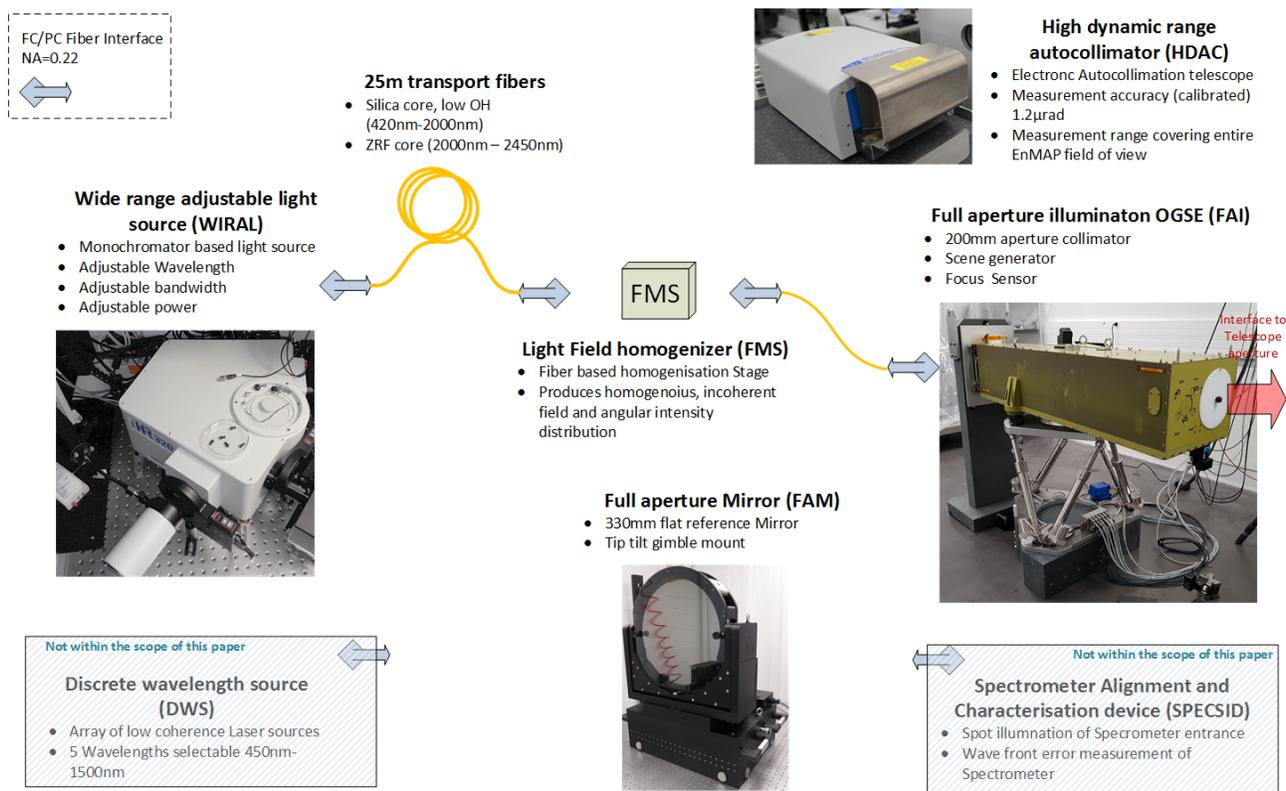
Figure 4 Overview of the general OGSE architecture. For a more detailed description of the individual Items c.f. Section 4 The Items DWS and SpecSid are shown for completeness only, they are not within the scope of this paper..
