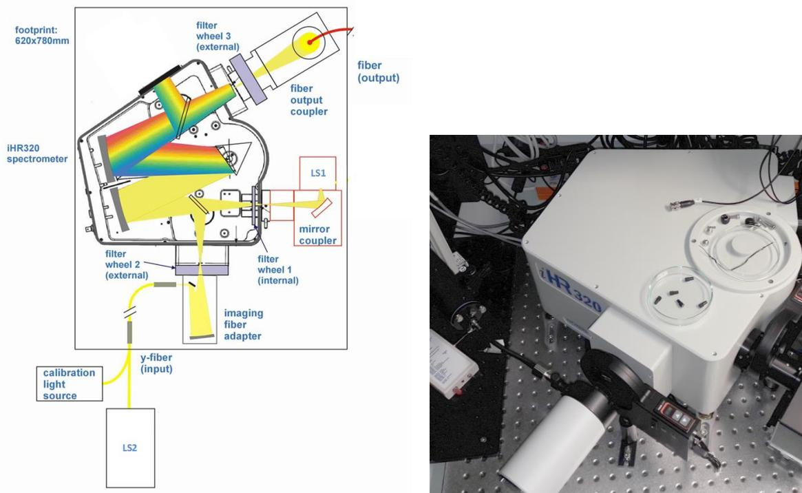
Figure 8 Wiral OGSE. Left: schematic overview of the architecture as designed by HORIBA, Right: Foto of the monochromator Setup
