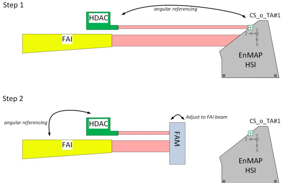
Figure 15 Schematic procedure to reference the FAI input beam with respect to the Telescope line of sight coordinate system CS\_TA#1
