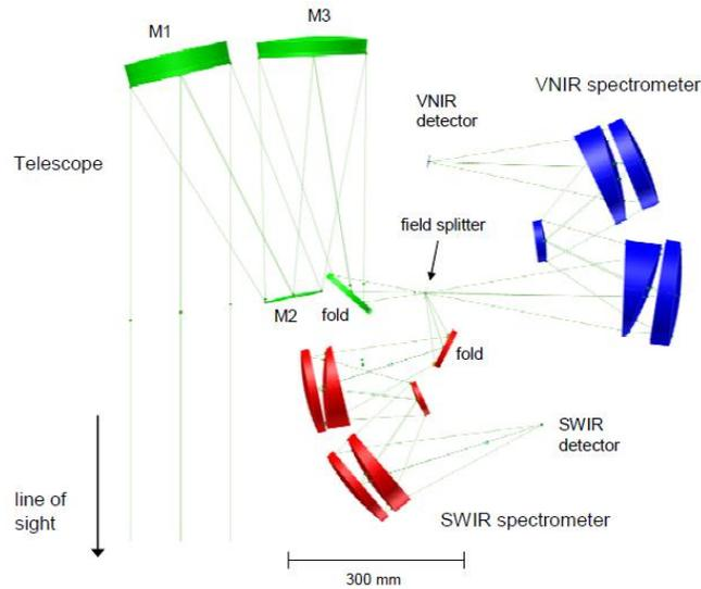
Figure 2 EnMAP HSI Optical beam path
