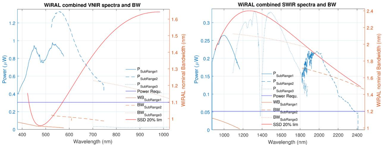
Figure 11 WIRAL wavelength ranges. Measured Power (light blue) and Spectral bandwidth defined as FWHM of the emitted spectrum (orange) are plotted against the minimum required power (solid blue) and the maximum required bandwidth (solid red)
