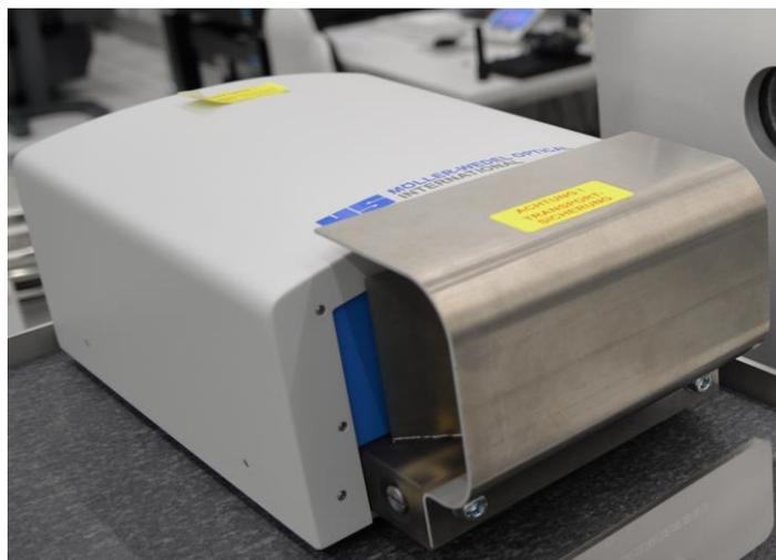
Figure 6 High dynamic range Electronic Autocollimator (built by Möller Wedel Optical GmbH)
