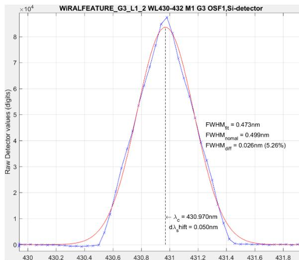
Figure 12 WIRAL bandwidth verification and wavelength drift characterisation based on Gas Cell reference lamp.
