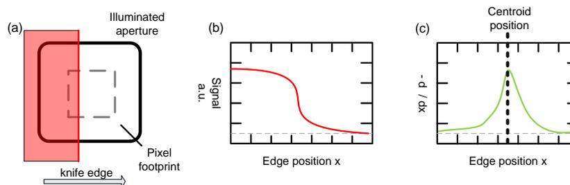
Figure 3 Determining the LoS of a pixel using a knife edge. (a) the image of a knife edge is scanned across the pixel of interest (b) the signal of the pixel as function of the knife edge position is the ESF of the imaging system including detector (c) the derivative of the obtained signal wrt the knife edge position yields the LSF again convoluted with the pixel size. The pixel LoS is defined as the centroid position of this function
