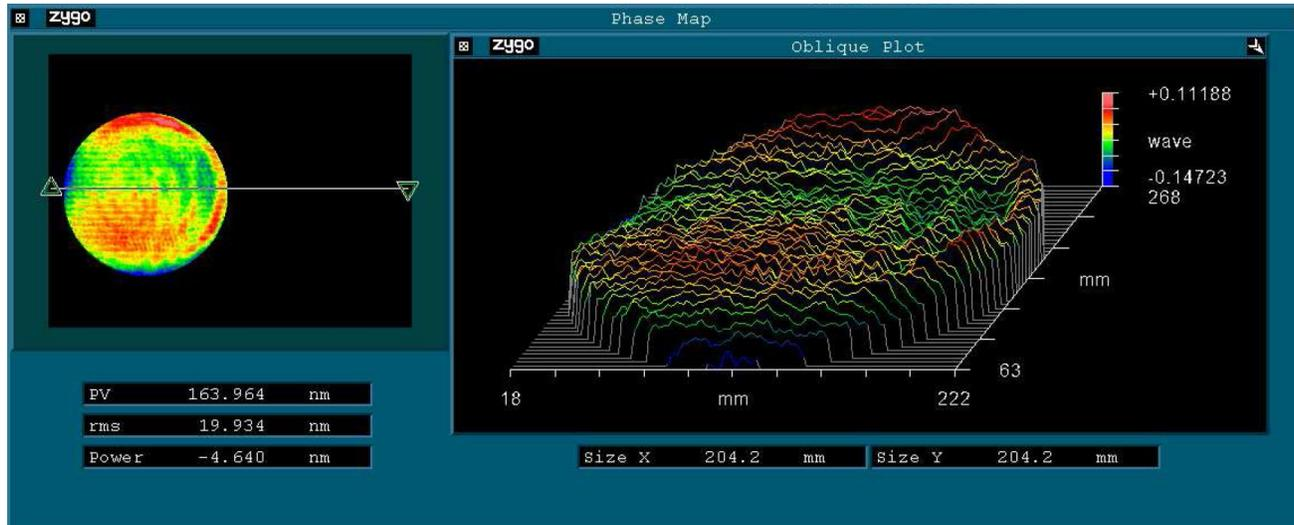
Figure 10 Wave front error map of the Collimator optical system for a central field point
