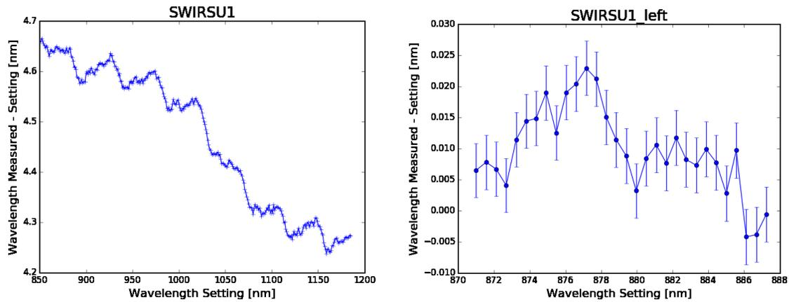
Figure 13 Wiral calibration results for one of the SWIR wavelength ranges. Measured Wavelength of light exiting the Wiral by a calibrated echelle spectrometer (GWU\_LambdaScan\_Spectrometer) before (left) and after (right) applying a calibration table. Please note the different x-scale of the two plots. (measurements performed by A. Baumgartner (DLR-IMF))
