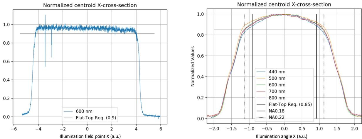
Figure 5 Intensity profiles at the FAI input Fiber port. Left: cut through the focal plane intensity pattern, Right: cut through the angular intensity pattern.
