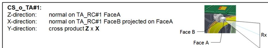
Figure 14 Operational definition of the Telescope Line of Sight coordinate system CS\_o\_TA#1 employing a mirror cube (TA\_RC#1) next to the telescope entrance
