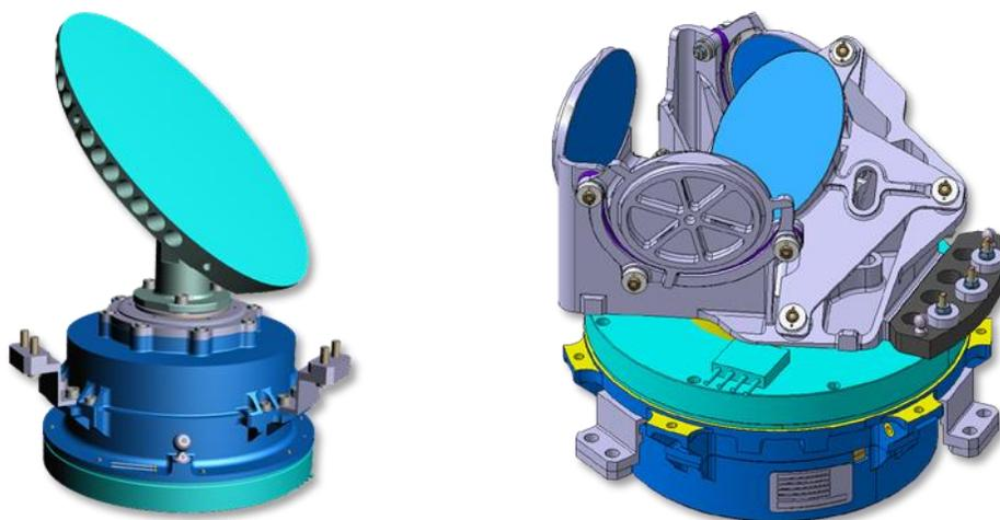
Figure 3. Scanner assembly (left) and Derotator assembly (right, courtesy of AMOS s.a [2]).
