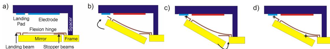
**Fig. 2.** Micromirror for multi-object spectroscopy: (a) Concept of the micromirror device. (b-d) A system of landing beam and stopper beams was introduced that provides uniform tilt-angle over the whole MMA.
