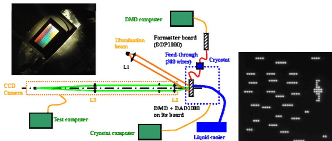
Fig. 7. (a) Schematic of the DMD space evaluation set-up; (insert: DMD image in the test chamber). (b) Typical MOS pattern (individual mirrors are ON)
