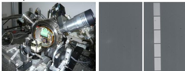
**Fig. 4.** Cryogenic set-up; functional testing of a micromirror array at 92K (0V and 90V applied)
