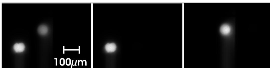
Fig. 6. CCD images corresponding to the image plane of the spectrograph. In the first image, two objects are present in the field of view, in the second and third image one out of two objects is selected, blocking completely the light of the other object. The projected object has a diameter of 50 $\mu$ m which corresponds to the size of a typical astronomical object in the focal plane of a telescope.
