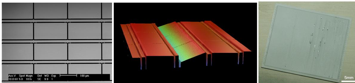
**Fig. 3.** (a) Frontside of the mirror chip with micromirrors of size 100 x 200 μm<sup>2</sup>. (b) One row is actuated, implementing the long slit mode. The fill factor is 97% along the slit. (c) Assembled MMA of size 25 mm x 22 mm with 200 x 100 micromirrors. Each micromirror is of size 200 x 100 μm<sup>2</sup>.
