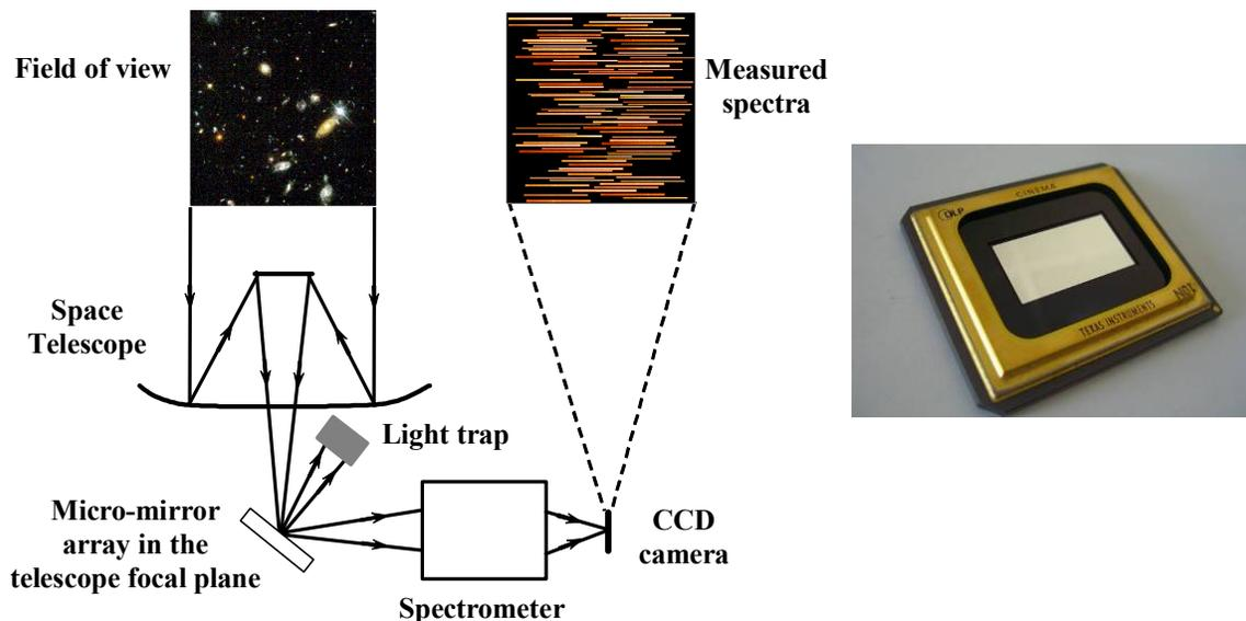
**Fig. 1.** Principle of a Multi-Object Spectrograph with a Micro-Mirror Array.
