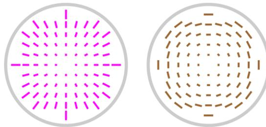
**Figure 5** The on-axis form for the polarization aberration (Left) when the p-component is greater than the s-component, (right) or, when the s-component is greater than the p-component. These forms are called diattenuation defocus or retardance defocus depending on which effect is being described.
