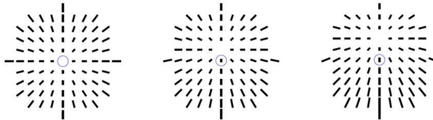
**Figure 7** Angle of incidence maps as the wavefronts of Figure 4 move off-axis. The patterns shift, but otherwise are unchanged. The ray through the center of each pattern (inside blue circle) is the chief ray for that field.
