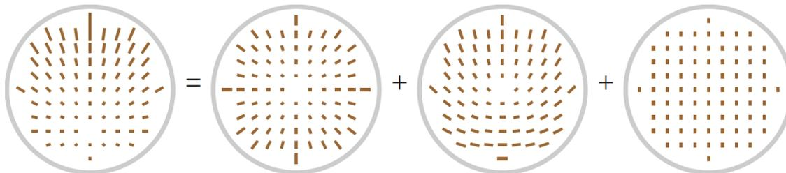
**Figure 9** The diattenuation map for an off-axis beam (left) has a quadratic variation along the y-axis. This map can be expressed as the sum of a quadratic variation, linear variation, and constant diattenuation. These are diattenuation defocus, diattenuation tilt, and diattenuation piston aberrations. Parallel components add, while crossed components cancel.
