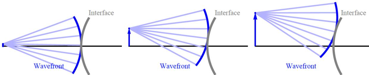
**Figure 6** Wavefronts from an on-axis and two off-axis objects incident on a spherical surface. All three cases are a spherical wavefront tangent to a spherical interface.
