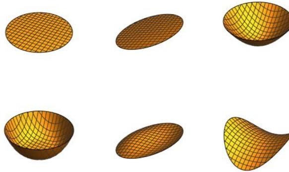
**Figure 3** The second and fourth order wavefront aberrations: piston, tilt, defocus, spherical aberration, coma, and astigmatism. Jim Wyant and I performed research to generalize these aberration forms to handle the diattenuation and retardance patterns in instrumental polarization.
