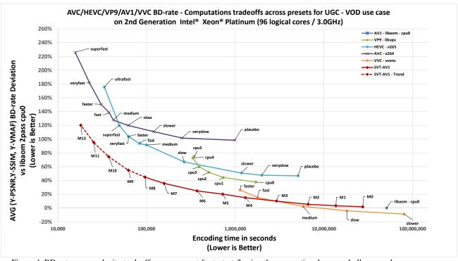
Figure 4. BD-rate vs complexity tradeoffs across preset for testset-3 using the conventional convex hull approach.
