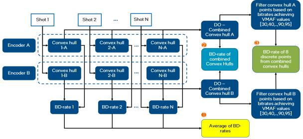
Figure 5. The three proposed approaches - "conventional" in yellow, "combined" in light blue and "restricted discrete" in green. DO stands for Dynamic Optimizer.
