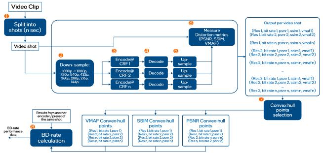
Figure 1. Shot-based encoding workflow.
