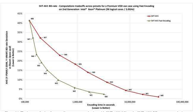
Figure 14. The impact of using fast encoding parameter selection with SVT-AV1 M8 on the SVT-AV1 BD-rate vs complexity tradeoffs across preset for testset-2.
