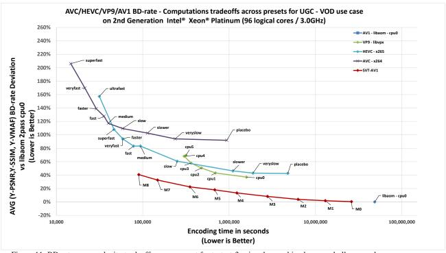
Figure 11. BD-rate vs complexity tradeoffs across preset for testset-3 using the combined convex hull approach.
