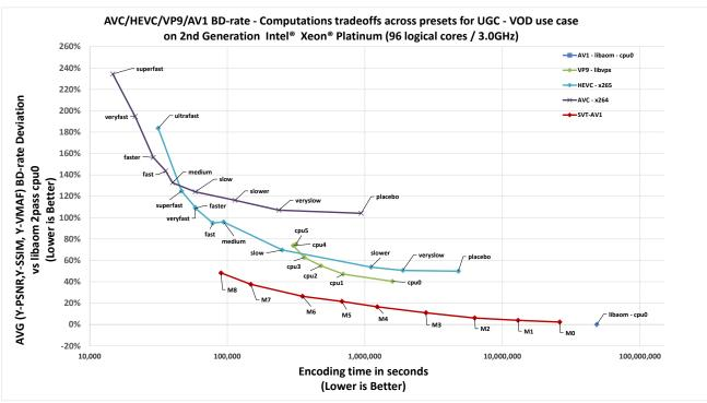
Figure 13. BD-rate vs complexity tradeoffs across presets for testset-3 using the restricted discrete convex hull approach.
