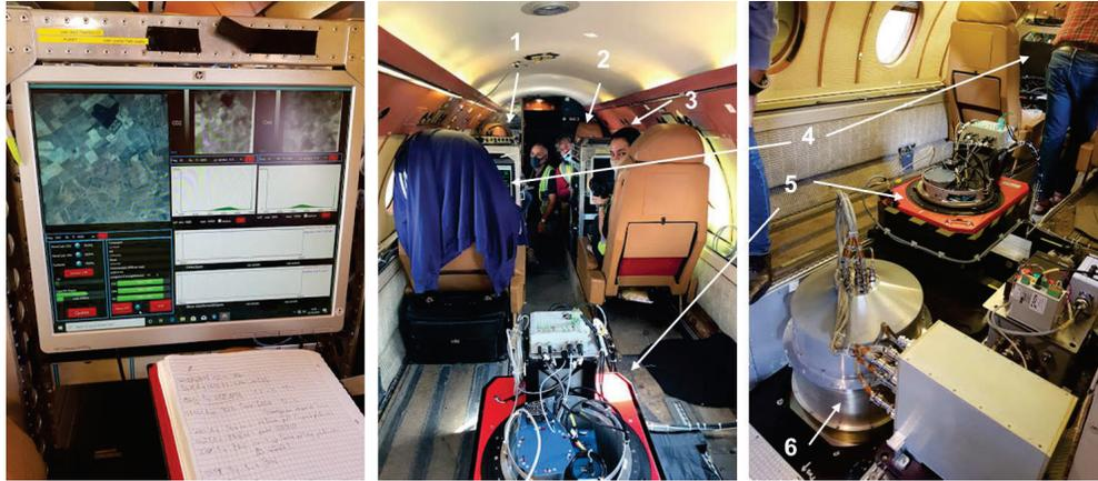
Figure 3. **Left:** NanoCarb user interface, seen from the NanoCarb operator seat. The image on the left is the visible image, while the two black and white images on the right are one thumbnail from the CO<sub>2</sub> and the CH<sub>4</sub> cameras. **Middle and right:** inside of the F20 1: Safire operator, 2: NanoCarb operator, 3: NanoCarb observer, 4: Spex operator, 5: GSM with the NanoCarb cameras, 6: SpexAirborne.
