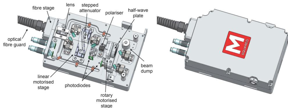
Figure 7. Mechanical drawings of the SolsTiS Beam Management Module.
