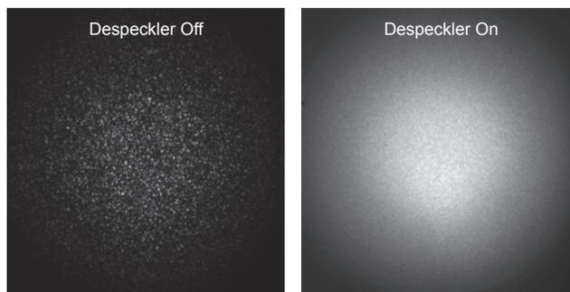
Figure 13. Images of the fibre output acquired when the Despeckler Module is off (left) and on (right).
