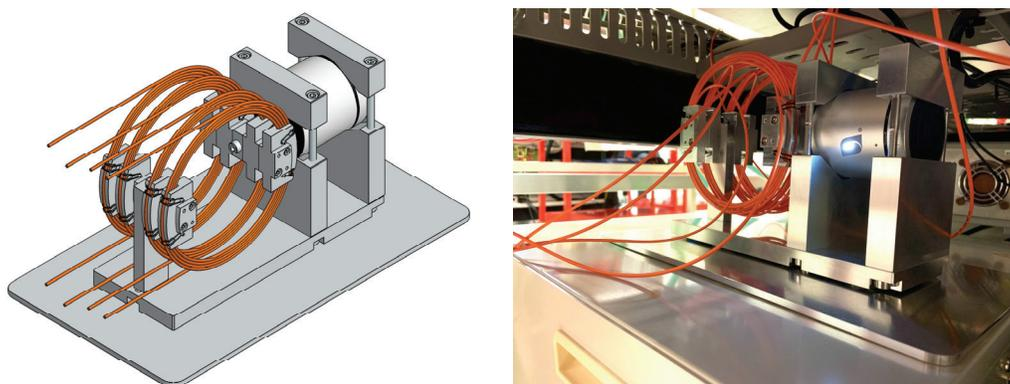
Figure 9. Mechanical drawing (left) and photo (right) of the despeckler module integrated to the design of AIT, VN and US laser systems, optimised to reduce the speckle from four optical fibres.
