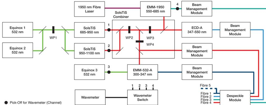
Figure 3. Schematic diagram of the VN Laser System design. WP: waveplate, VPPO: variable pump pick-off, VIRPO: variable infrared pick-off.
