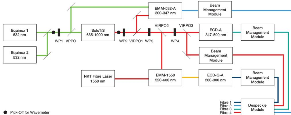
Figure 1. Schematic diagram of the AIT Laser System design. WP: waveplate, VPPO: variable pump pick-off, VIRPO: variable infrared pick-off.
