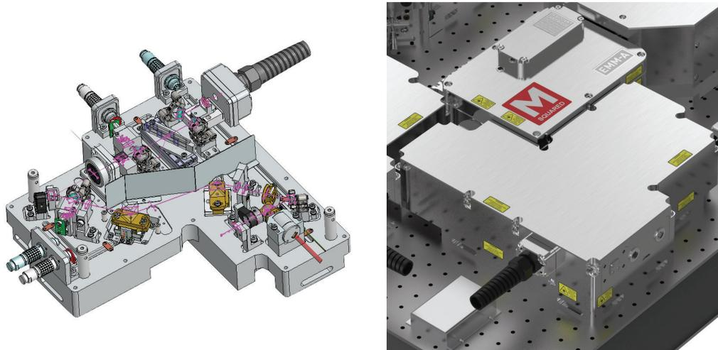
Figure 8. Mechanical drawing (left) and render (right) of the beam management module for automated ECD and EMM laser modules.
