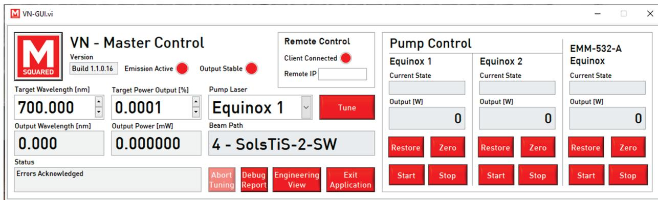
Figure 16. Example of the master control interface provided for each laser system, giving full access to wavelength, relative power, absolute power, power readout among many more features.
