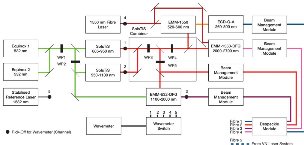
Figure 5. Schematic diagram of the US Laser System design. WP: waveplate, VPPO: variable pump pick-off, VIRPO: variable infrared pick-off.
