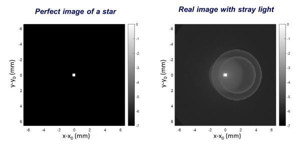
Figure 2: (left) Perfect image of a star. (right) More realistic image of that star when considering also the stray light
