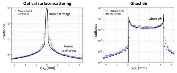
Figure 8: Profile of the scattering by the lenses surface roughness (left) and profile of a single ghost (eb). The blue dots show the experimental results, the ray tracing is overlayed to show the reverse engineering capabilities for scattering or comparison with theory for the ghosts
