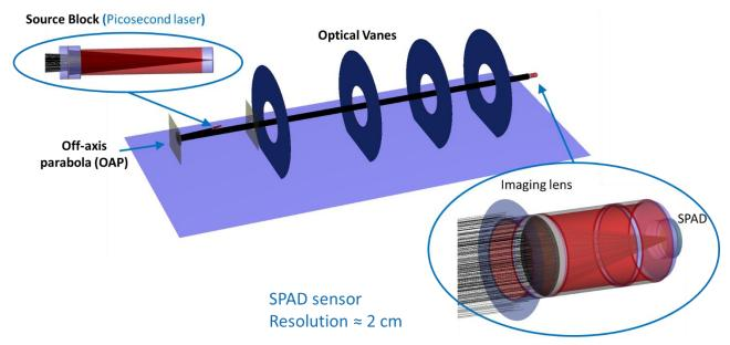
Figure 11: Sketch of the interior of the calibration device with the spad detection system replacing the FLEX instrument, used fo timeof-flight characterization and validation of the facility
