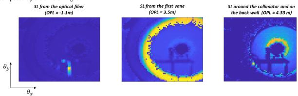
Figure 12: Illustration of stray light pattern arriving at the spad detector at different moments, showing different stray light contributor
