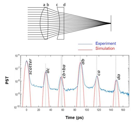
Figure 5: (Top) Decomposition of the stray light by the time of flight, considering the spatially integrated stray light as defined by the point source transmittance function (PST), for ghost in the optical system shown on the bottom illustration. Experimental and theoretical results are displayed.
