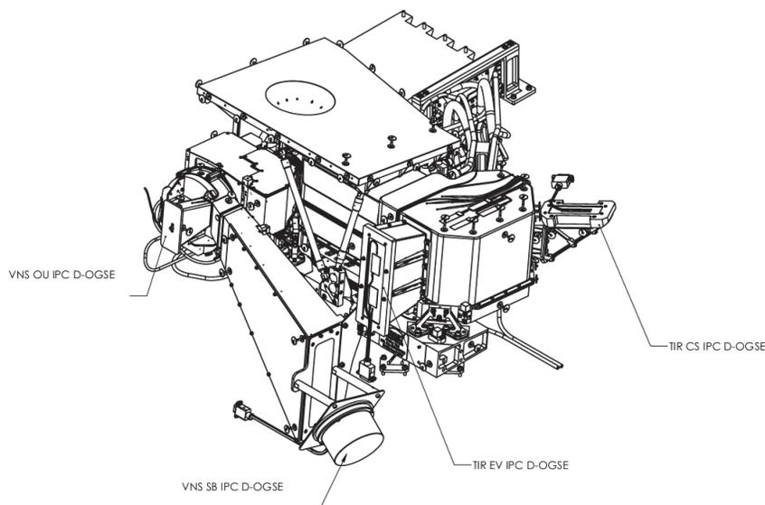
Figure 10. MSI Instrument with all Instrument Performance Check OGSEs attached.
