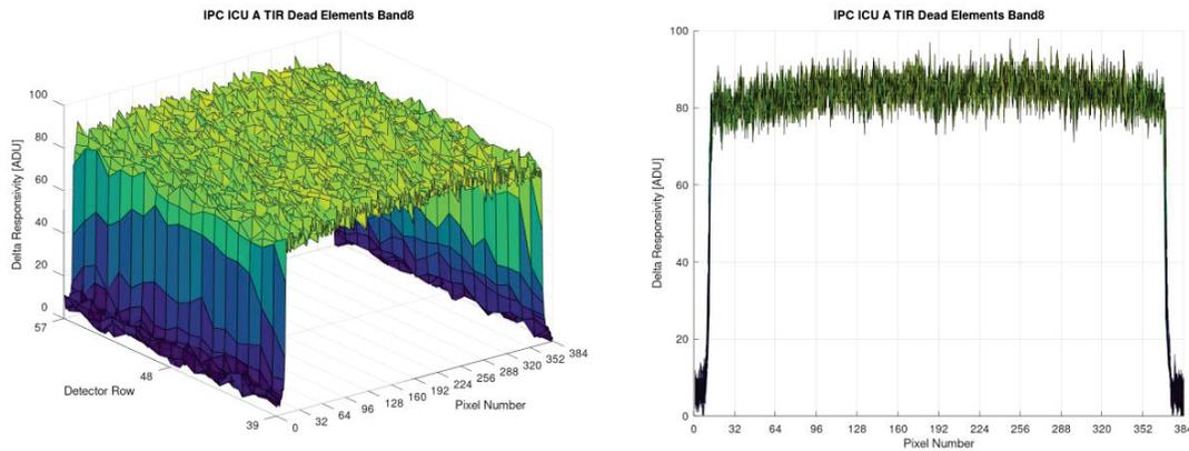
Figure 20. TIR Dead Element response map Band8 during post MSI integration on Platform IPC.
