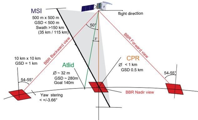
Figure 3. EarthCARE observation concept. The footprints of the nadir-pointing CPR and MSI, the 3° backward-looking ATLID, and the three BBR views
