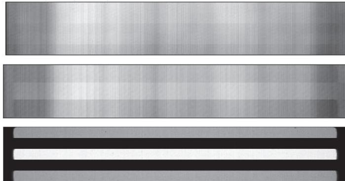
Figure 18. IPC processing for TIR dead element evaluation. (From top to bottom TIR RAW HOT, TIR RAW COLD and Responsivity map)
