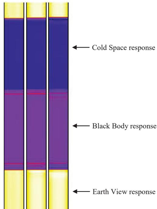
Figure 16. TIR calibrated response measurements for spectral bands 7, 8 and 9 in false coloring.
