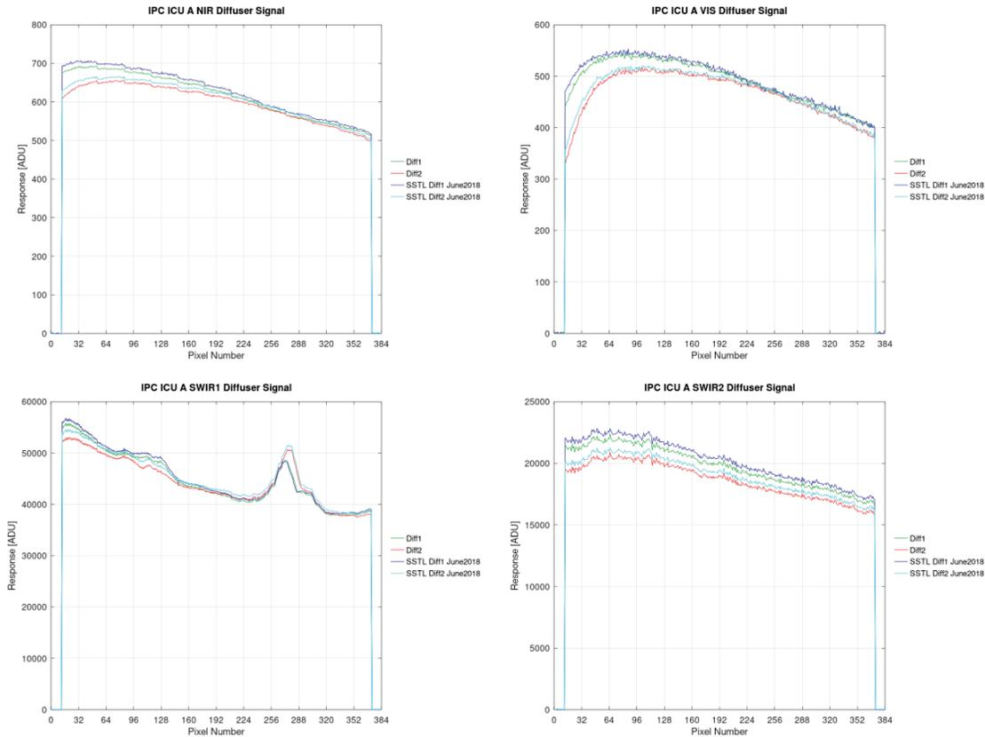
Figure 14. VNS response measurements for spectral bands VIS, NIR, SWIR-1 and SWIR-2 during post MSI integration on Platform IPC in comparison to supplier level measurements during TBTV campaign.
