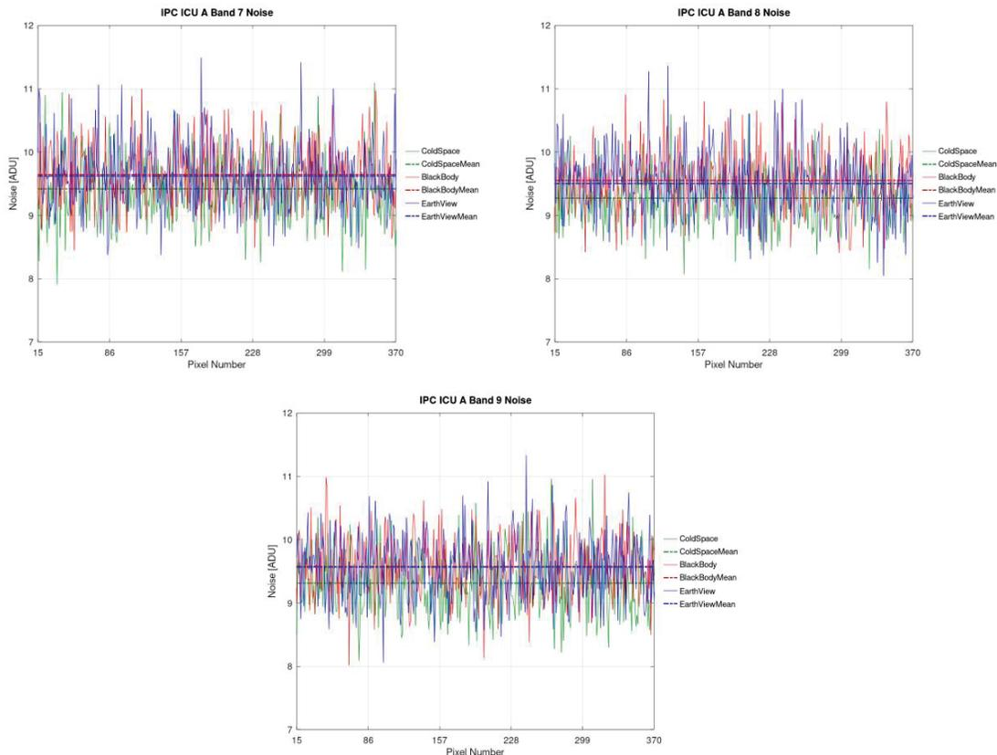
Figure 13. TIR Noise measurements for spectral bands 7,8 and 9 during post MSI integration on Platform IPC.
