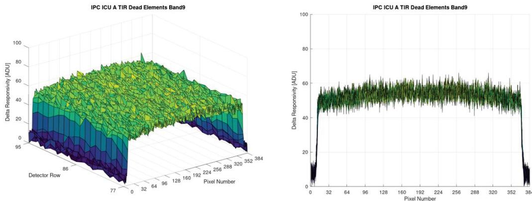
Figure 21. TIR Dead Element response map Band9 during post MSI integration on Platform IPC.
