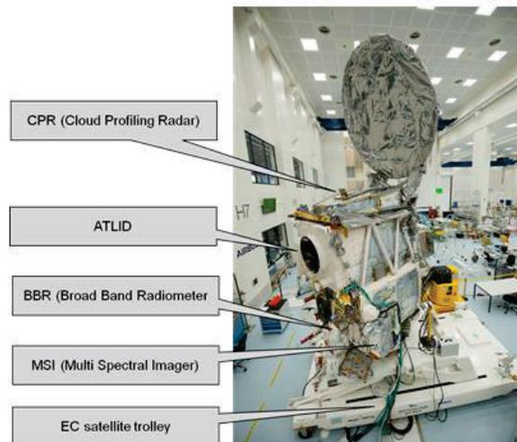
Figure 4. EarthCARE satellite with all instruments integrated in Airbus Friedrichshafen cleanroom.
