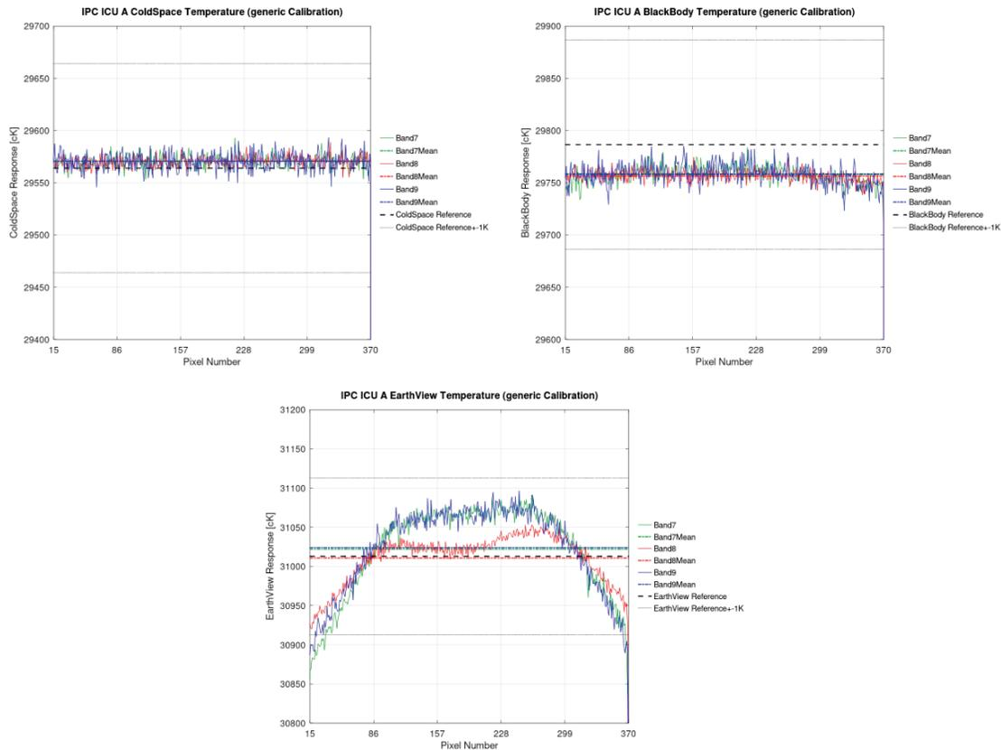
Figure 17. TIR calibrated response for spectral bands 7,8 and 9 in centi kelvin for all view scenes during post MSI integration on Platform IPC.
