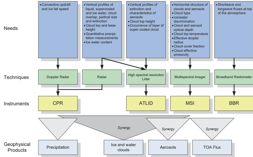
Figure 2. Summary of measurement needs, measurement techniques and the related EarthCARE instruments. The EarthCARE sensors as a complement will produce a set geophysical product for which again synergy is needed to perform the process studies of interest
