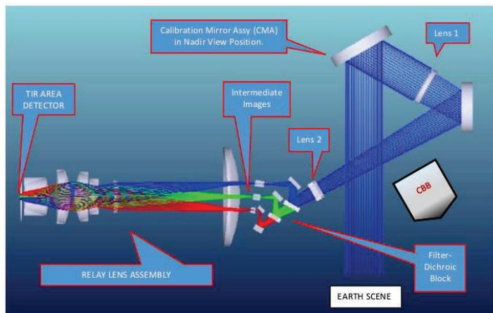
Figure 9. TIR two-stage optics. Telescope (Lens 1 and Lens 2) and filter-dichroic block form three spectrally filtered intermediate images which are de-magnified onto the area detector using the Relay lens. For simplicity, the rotating calibration mirror is shown fixed in the “nadir view” position, and the cold-space port is omitted. The CBB position is indicated.
