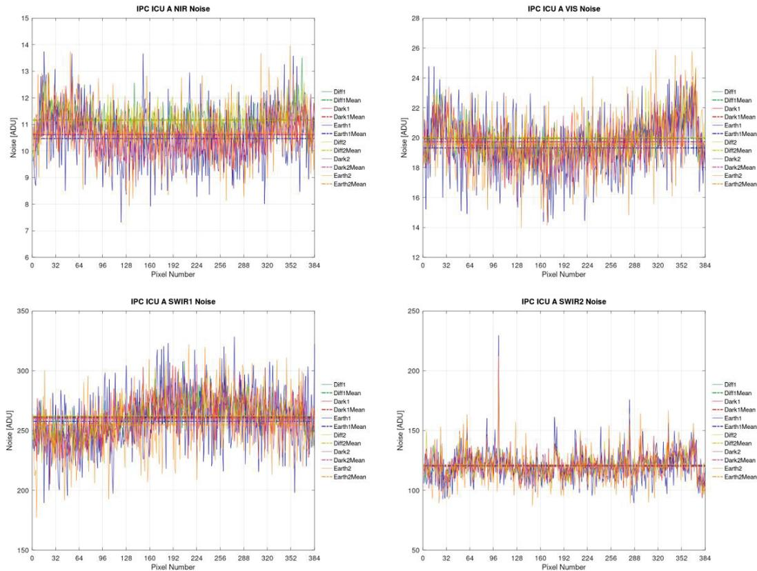
Figure 12. VNS Noise measurements for spectral bands VIS, NIR, SWIR-1 and SWIR-2 during post MSI integration on Platform IPC.
