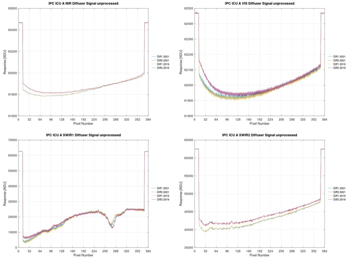
Figure 15. VNS unprocessed response measurements for spectral bands VIS, NIR, SWIR-1 and SWIR-2 during post MSI integration on Platform IPC in comparison to post MSI Hardware modification IPC.
