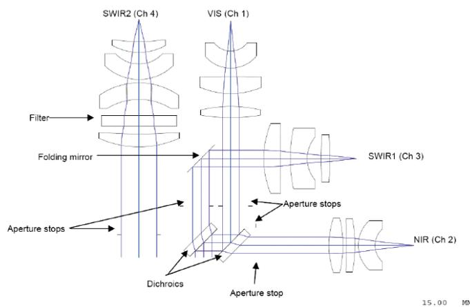
Figure 8. VNS Optical Schematic. SWIR-2 (left) has its own entrance aperture, whilst VIS / NIR / SWIR-1 share a common aperture and receive their light via dichroic filters.
