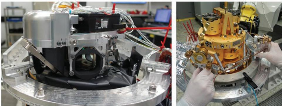
Figure 10. METimage cryogenic subsystem first flight model. Warm optical assembly (left) and cryogenic imaging assembly (right).
