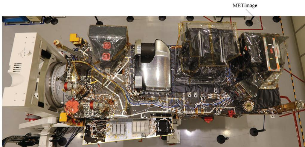
Figure 4. METimage engineering model on-board MetOp-SG satellite A (courtesy Airbus Defence & Space SAS).
