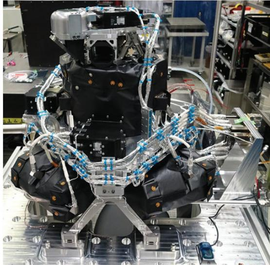
Figure 9. METimage cryogenic subsystem first flight model.
