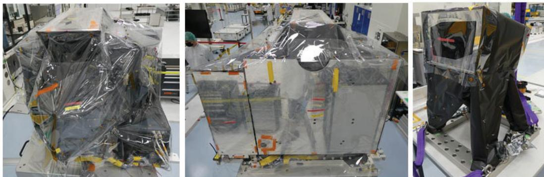
Figure 3. METimage engineering model. Optical head and external electric assembly (left, centre) and solar calibration device baffle (right) with contamination protection covers on the transport adapters.
