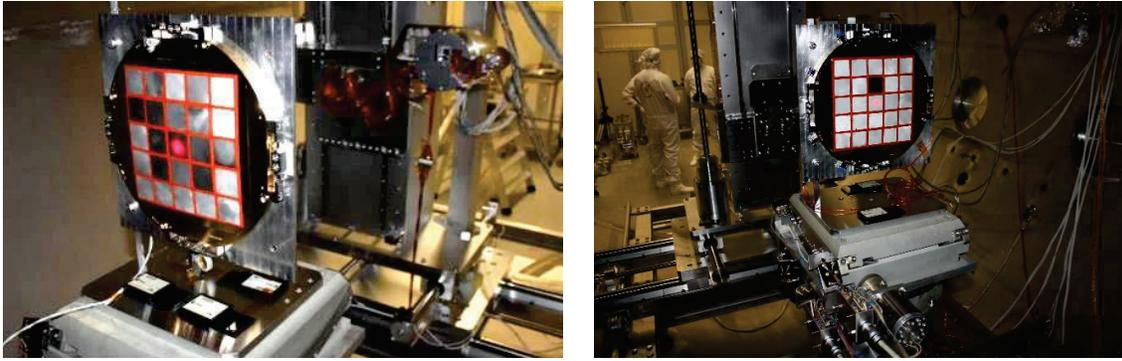
Figure 2 SVOM-MXT-MOP optics in the PANTER vacuum chamber, view from the source toward the detector: (left) the Flight Model (FM), and (right) the Flight Spare (FS) models are shown.
