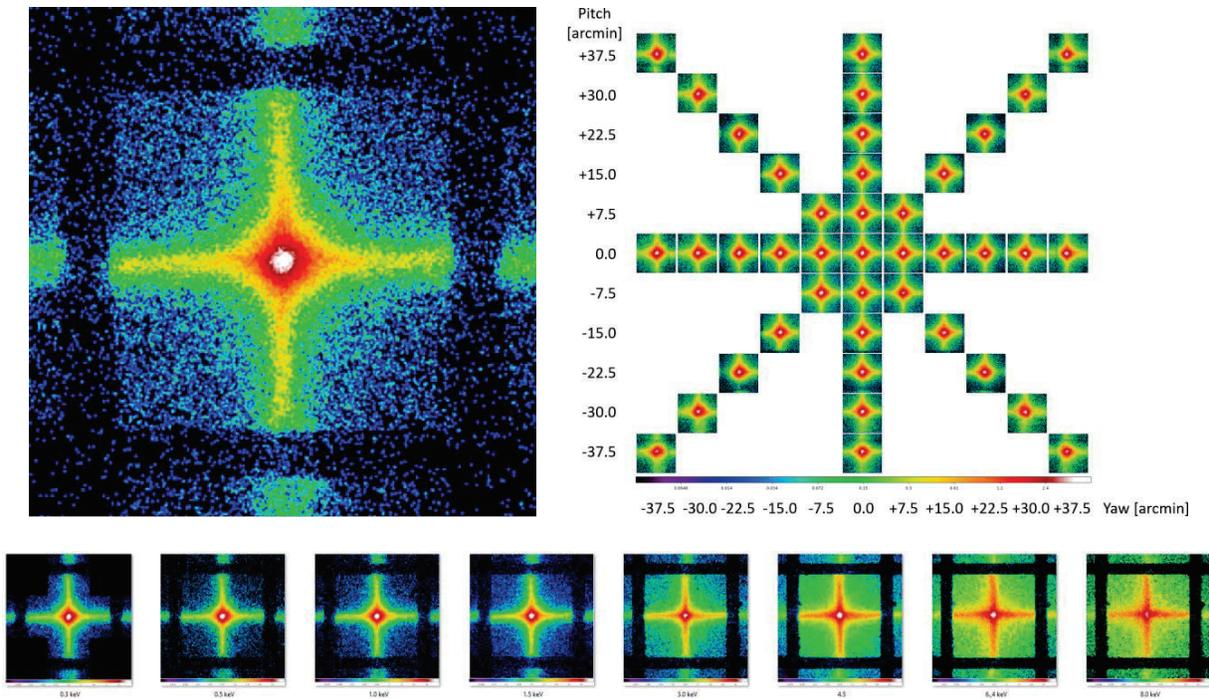
Figure 3 Measurements of the MXT-MOP-FM at Al-K (1.5 keV): (top left) a grid of  $3 \times 3$  TRoPIC images combined to study the cross arms of the PSF in detail, (top right) a so-called focal plane map obtained to study variation of the PSF and efficiency of the optic on-axis as well as for a grid of off-axis angles. (bottom) the PSF as a function of energy is shown from left to right C-K, O-K, Cu-L, Al-K, Ag-L, Ti-K, Fe-K, Cu-K.
