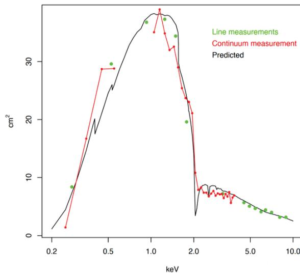
Figure 9 This plot shows the effective area of the SVOM-MXT-FM telescope as measured in PANTER during the performance tests: in green the effective area measurements at the characteristic lines of the X-ray source target elements available at PANTER, in red the continuum flux measurements and in black the effective area model prediction (image taken from [10]).
