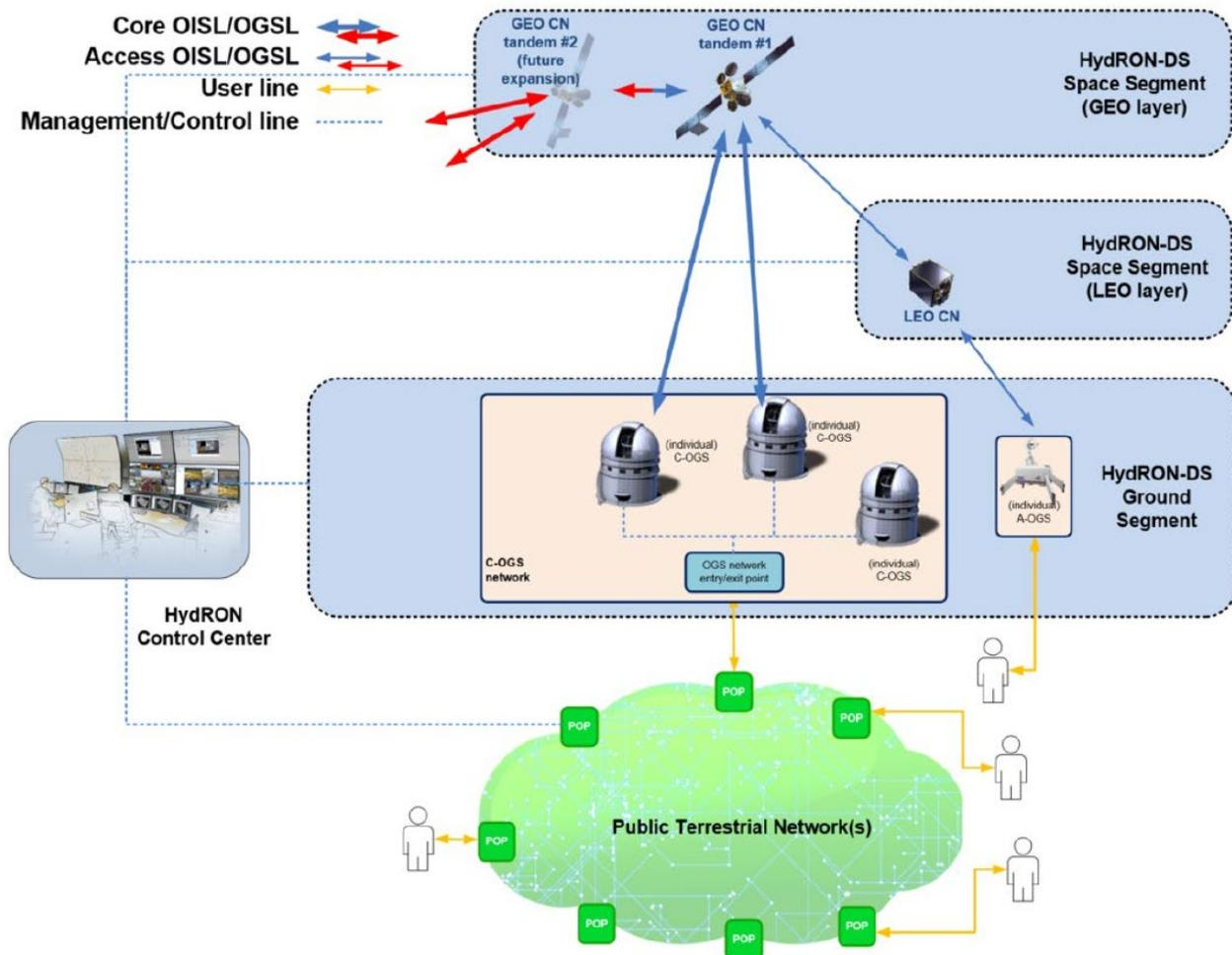
**Figure 15: Technical Baseline of HydRON DS Proposal. The Space Segment consists of two co-located GEO payloads, a payload in LEO orbit as well as of Ground Segment with a total of four OGS. The HydRON Control Centre orchestrates all the HydRON DS elements, as well as the interface with users for service demonstration**
