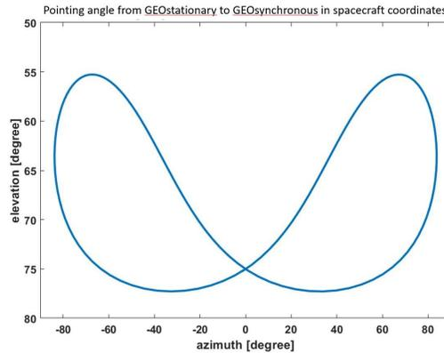
**Figure 10: Required pointing angle from GEOstationary node at 16°E to cover a GEOsynchronous node at 46°E.**
