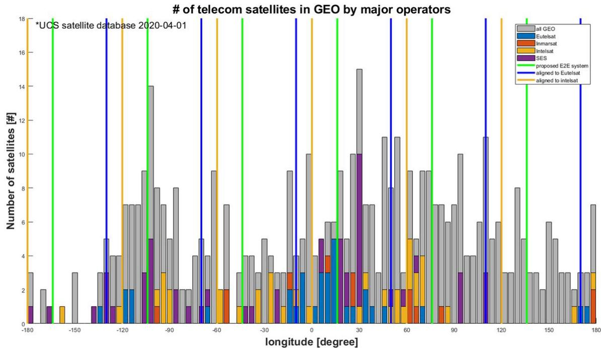
**Figure 4: Satellite orbital slots in GEO per major operator**
