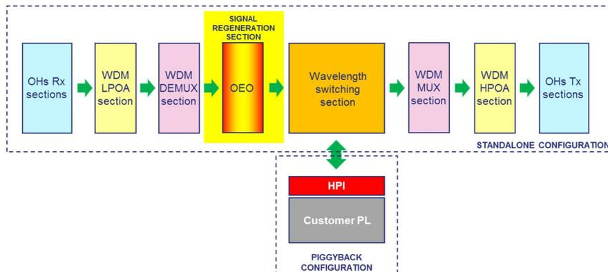
**Figure 13: HyDRON hybrid payload functional architecture**
