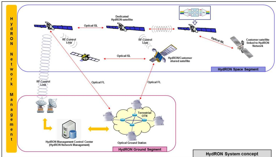
**Figure 11: HydRON top level system concept**
