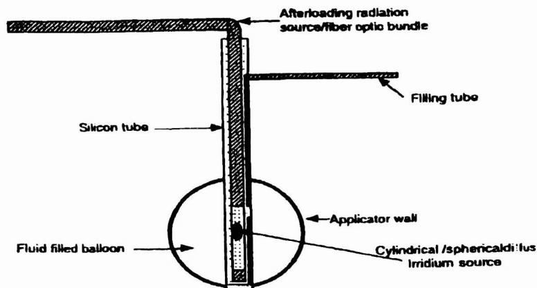
Figure 3. An indwelling balloon applicator for brachy and photodynamic therapy.
