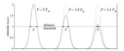
Figure 1. Schematic illustration of how one can overcome the diffraction limit by taking advantage of the well-defined ablation threshold
