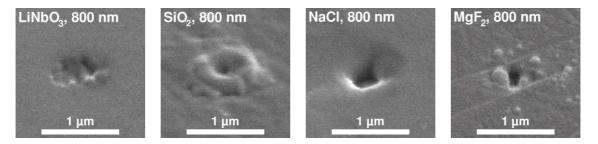
Figure 4. SEM images of sub-micrometer ablation results on different materials
