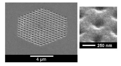
Figure 5. An example of a periodic nanostructure (with a defect cavity in the center) fabricated in a sapphire crystal with femtosecond laser pulses (*left*). On the *right side* an enlarged fragment of a single hole is shown.
