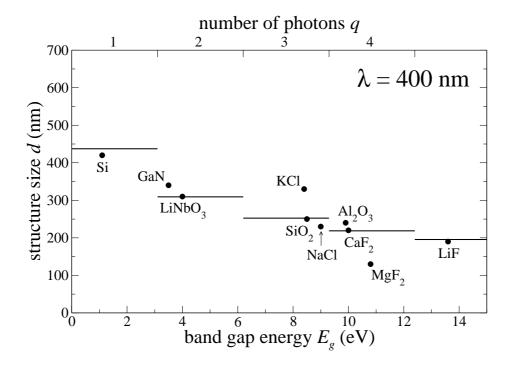
Figure 7. Structure sizes for a laser wavelength of 400 nm on materials with different band gap energies
