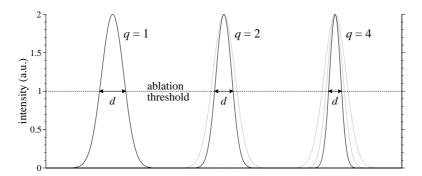
Figure 3. Effective beam profile and ablation hole diameter for materials where q = 1, 2 and 4 photons are needed for each ionization process
