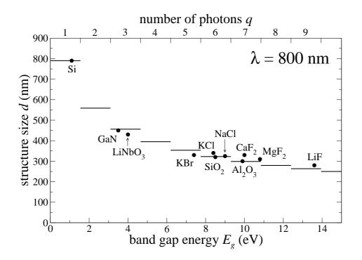
Figure 6. Structure sizes for a laser wavelength of 800 nm on materials with different band gap energies
