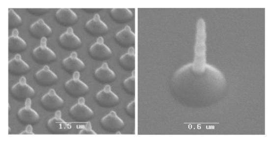
Figure 2. SEM images of an array of nanojets fabricated in a gold film with femtosecond laser pulses (*left*) and a single nanojet in detail (*right*)
