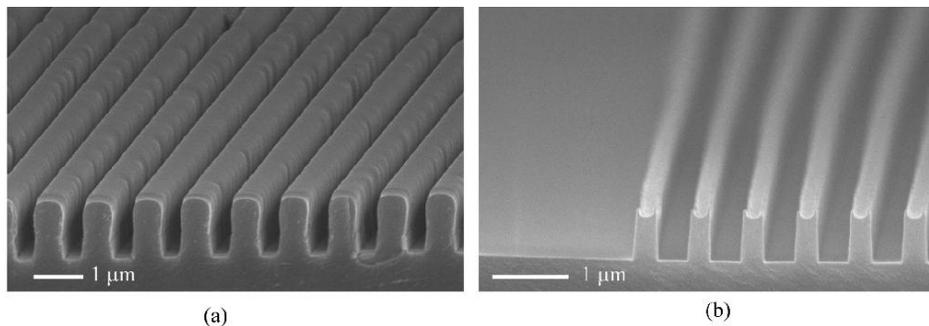
Figure 3: a) UV cured linear binary grating with a feature size of  $0.5 \mu\text{m}$  for spectroscopic applications and b) UV cured “Bragg” diffractive lens structure.
