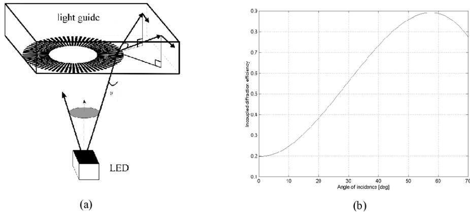
Figure 9: a) Light incoupling geometry with radial light coupler, b) theoretical diffraction efficiency of the grating as a function of angle of incidence.
