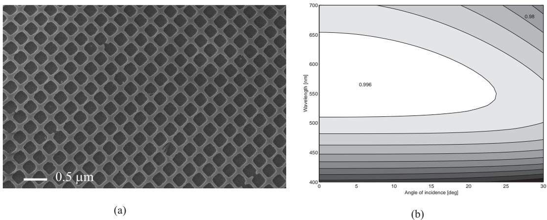
Figure 7: a) Antireflective binary crossed grating is SiO<sub>2</sub> b) theoretical transmission as a function of wavelength and the incidence angle.
