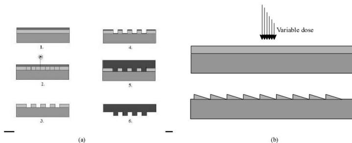
Figure 1: a) Binary grating manufacturing: 1. Resist spinning on the substrate, 2. direct electron beam, laser writing, or holographic recording, 3. development, 4. evaporation of conductive layer, 5. nickel electrolysis, and 6. nickel separation (1<sup>st</sup> generation shim). b) principle of direct writing of continuous grating with a variable dose to analogue resist (phases 2 and 3 are shown).
