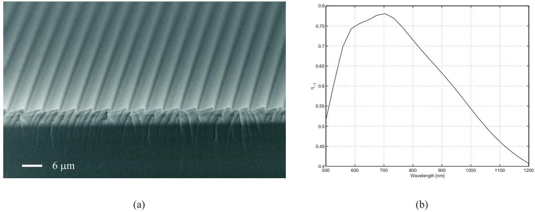
Figure 6: a) Blazed grating structure, grating period 6 μm, grating depth 1.1 μm and refractive index n=1.54 b) Theoretical diffraction efficiency as a function of wavelength.
