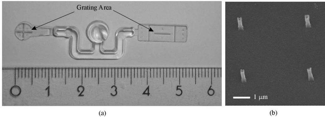
Figure 4: a) Micro injection molded plastic piece (centimeter unit is seen). b) Micro-injection molding resolution test with a feature size of  $<300\text{ nm}$  and with a depth  $>300\text{ nm}$ .
