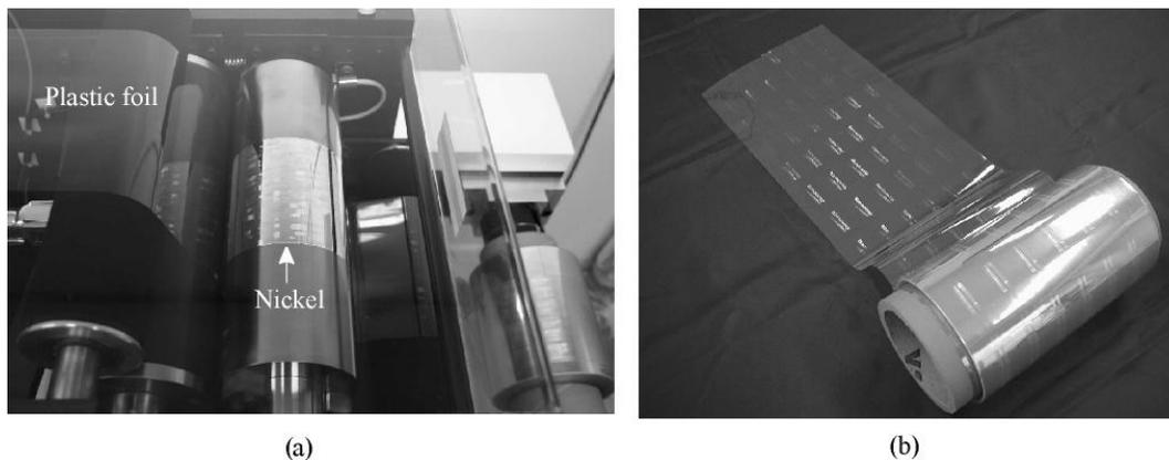
Figure 5: a) Reel-to-Reel production of diffractive optics. Nickel tool is wrapped around the cylinder that is heated and pressed against the plastic foil. b) (Small) roll of the material embossed with R2R production.
