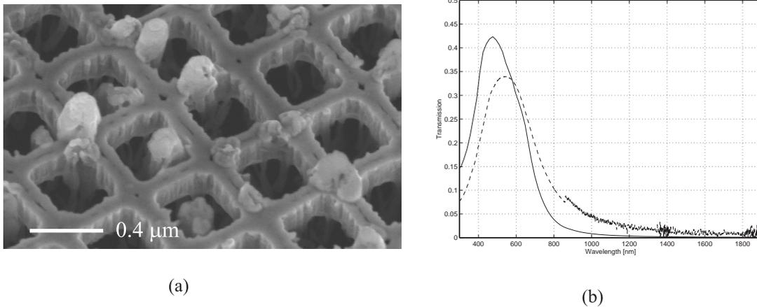
Figure 8: a) Iridium grid grating for infrared rejection b) experimental (dashed line) and theoretical (solid line) transmission of such a grating as a function of wavelength.
