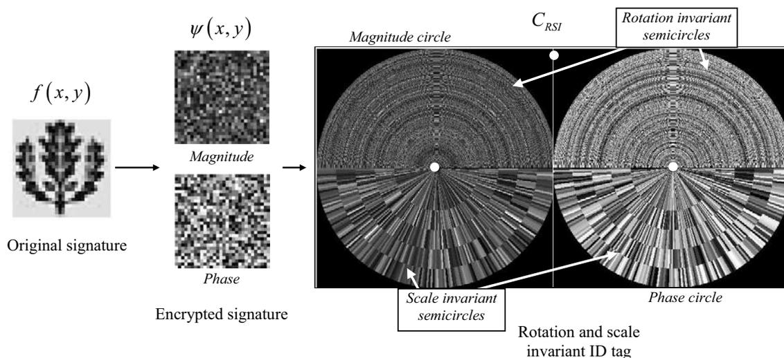
Fig. 2. Synthesis of a distortion (rotation and scale)-invariant ID tag.
