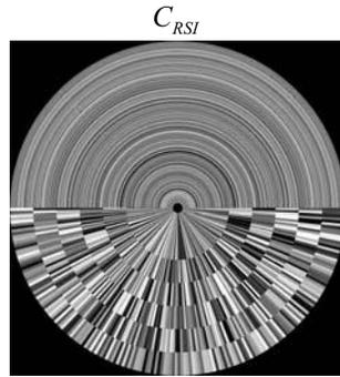
Fig. 5. Distortion invariant ID tag built from the phase-only encrypted signature. The grayscale encoded information is only noticeable in the NIR spectral band.
