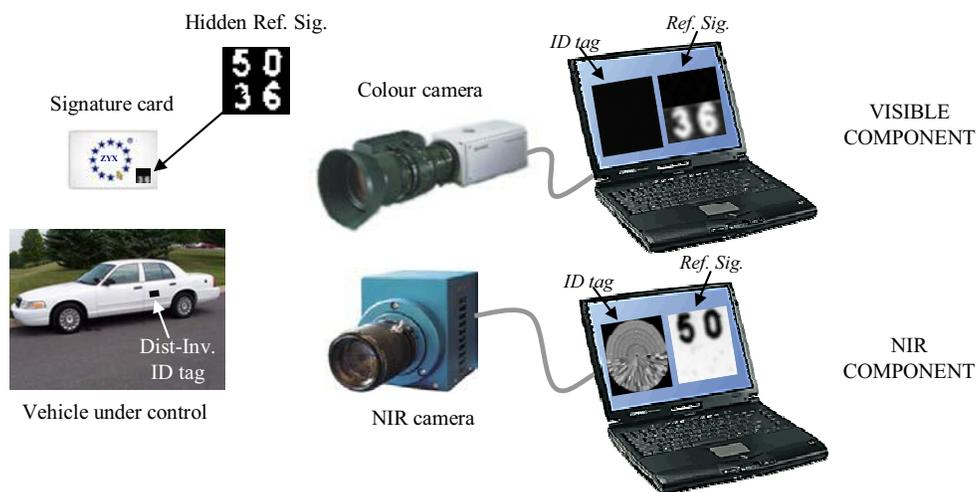
Fig. 4. Example of the two-spectral proposal. The distortion invariant ID tag, which is built from the phase-only encrypted signature, is located on a sidewall of a vehicle. On the one hand, the grayscale encoded information is only noticeable in the NIR spectral band but not in the visible component. On the other hand, both visible and NIR components of the image on the card permit to obtain the whole reference signature.
