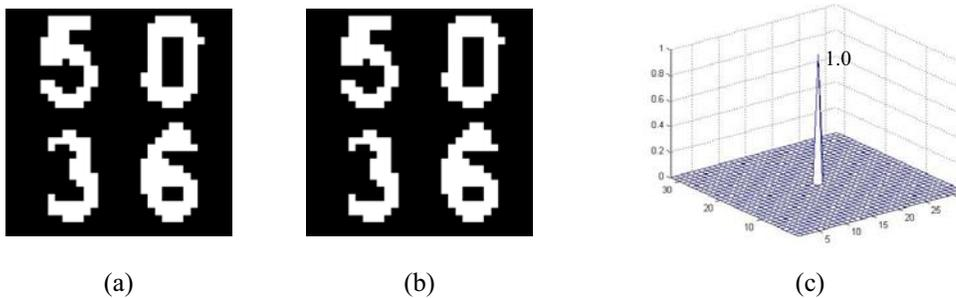
Fig. 6. (a) Signature retrieved from the distortion-invariant ID tag. (b) Reference signature  $f(x, y)$  obtained from the appropriate combination of the visible and NIR components (Eq. 3). (c) Output ( $ac$ ) of the verification system that leads to a positive identification.
