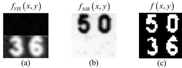
Fig. 3. (a) Visible and (b) NIR spectral components of the reference signature. (c) Complete signature that results from the logical operation of Eq. (3) applied to the visible and NIR binarized components.
