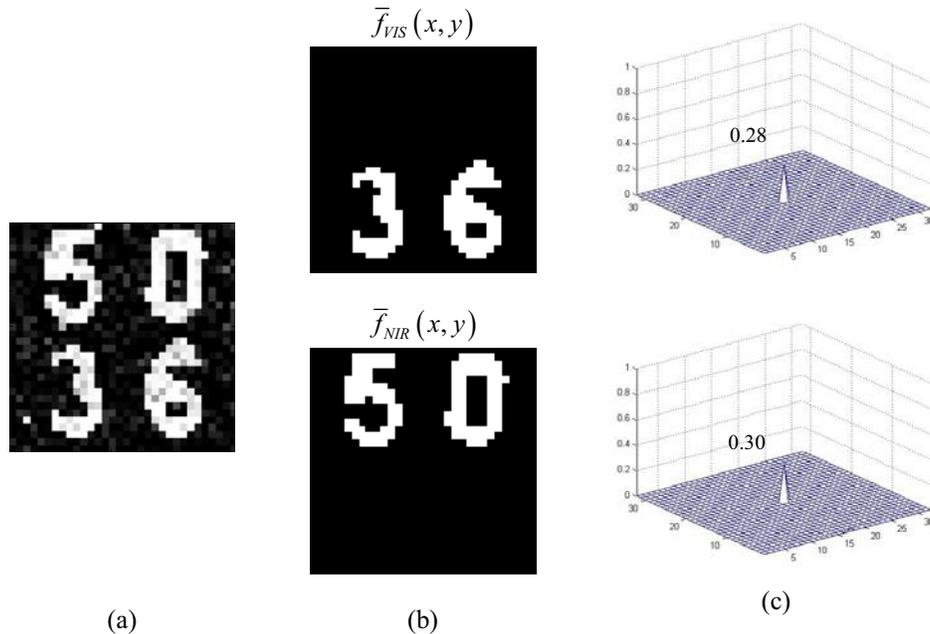
Fig. 9. (a) Signature retrieved from the phase-only distortion-invariant ID tag of Fig. 5. (b) Reference binarized signatures obtained from one single spectral channel, either the visible (top) or the NIR (bottom) spectral bands after being processed to obtain a binary image. (c) Outputs ( $cc/ac$ ) of the verification system that leads to a negative result for the visible (top) and NIR (bottom) components.
