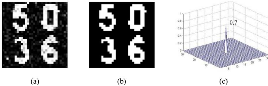
Fig. 7. (a) Signature retrieved from the phase-only distortion-invariant ID tag of Fig. 5. (b) Reference signature  $f(x, y)$  obtained from the appropriate combination of the visible and NIR channels (Eq. 3). (c) Output ( $cc/ac$ ) of the verification system that leads to a positive identification.
