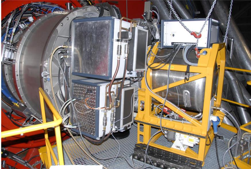
Figure 9: LUCIFER (left) with an auxiliary cryostat attached (right). The aux. cryostats rails on the bridge are also visible.
