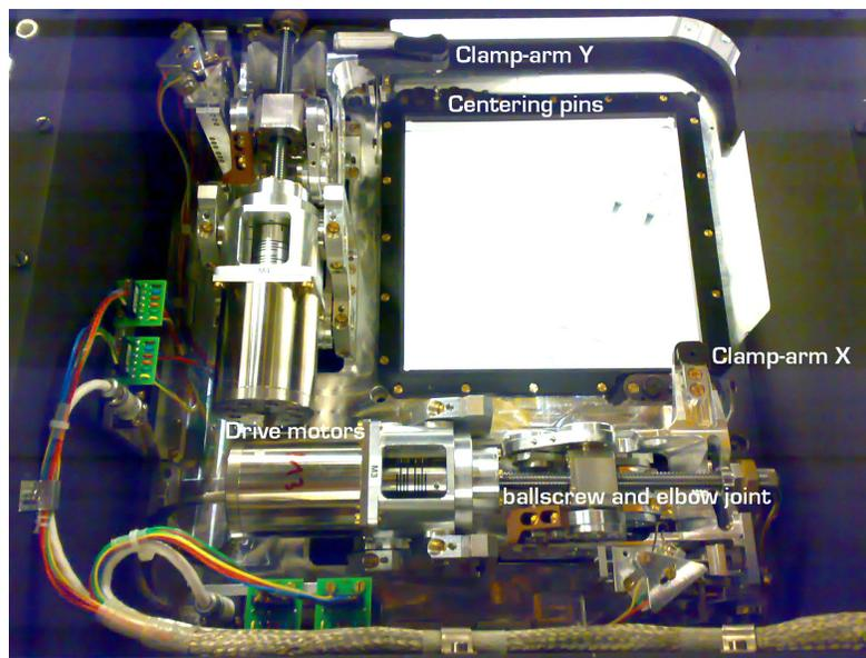
Figure 4: The Focal Plane Unit inside the cryostat. The black frame defines the FOV when no mask is present.
