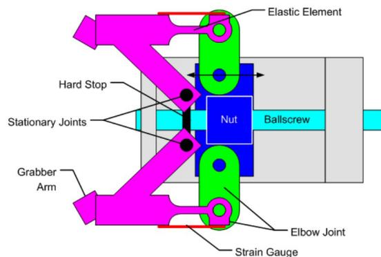
Figure 5: Schematic drawing of the grabber in dead center configuration. Moving slightly to the left selflocks the grabber.
