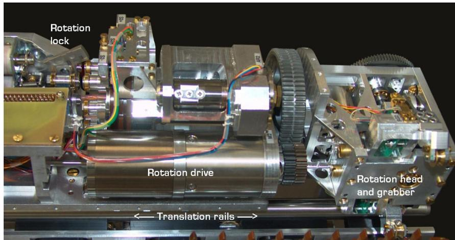
Figure 6: The Mask Handling Unit in storage position
