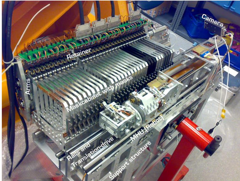
Figure 2: Storage and Mask Handling Unit during maintenance outside the main cryostat. MHU rotation head is in storage position with the grabber open, ready to grab a mask. The Focal Plane unit is not visible in this image. The silver mask frames have meanwhile all been replaced with blackened ones.
