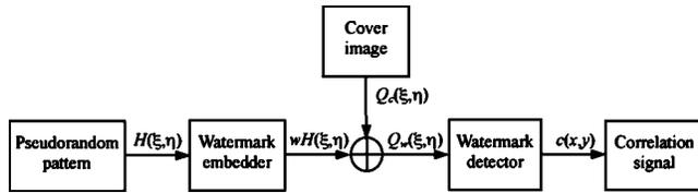
Fig. 1 Proposed correlation-based watermarking scheme.
