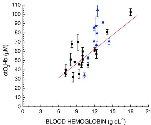
**Fig. 3** Absolute comparison between invasively measured hemoglobin and DOS measured  $\text{ctO}_2\text{Hb}$ . Nontransfused as well as transfusion infants are shown (squares). Error bars represent the SD of the results from repeated individual measurements (17 subjects, 34 measurements). The solid line is an error-weighted ( $r=0.83, p<0.0001$ ) fit involving the initial measurements on all 17 subjects. Squares represent the post-transfusion measurements (but were not included in the fit).
