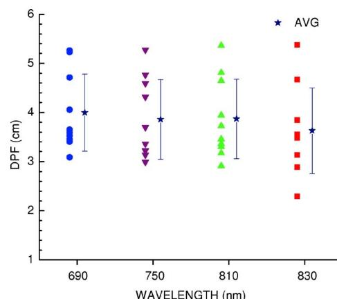
**Fig. 5** Plot of the distribution of calculated DPF values from the ten transfused subjects for each wavelength. The stars and error bars next to each column represent the population average for that particular wavelength. Note the variation is approximately 20% for each wavelength. The source-detector separation was taken to be the mean of the four distances (15 mm).
