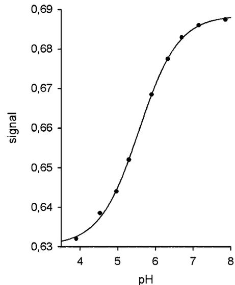
**Fig. 5** Calibration curve of the 30% APTS sensing capillary, the response curve of which is shown in Fig. 4.
