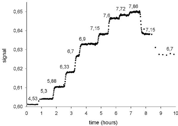
**Fig. 6** Response curve of a 10% APTS sensing capillary. The numbers in the graph are the pH values of the McIlvaine buffers.
