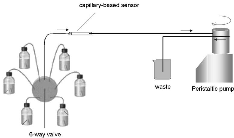
Fig. 2 Setup of the fluidic system for the characterization of pH-sensing capillary.
