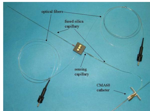
**Fig. 9** Particular of the fluidic system for the microdialysis measurements, showing the flow cell, the optical fibers, and the CMA 60 catheter.
