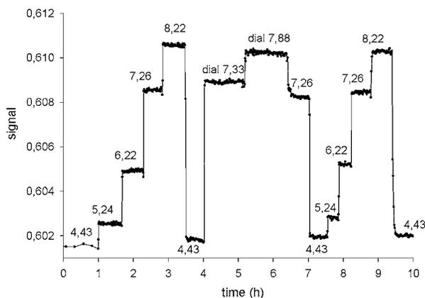
**Fig. 10** Effect of a 3-h exposure of the pH sensing capillary to dialyzed blood; the pH values of the buffer and of the dialyzed blood are shown.
