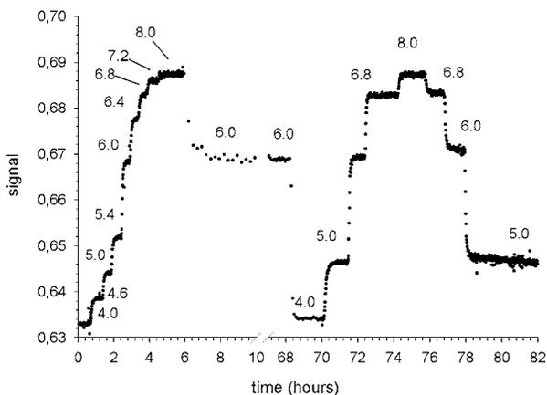
**Fig. 4** Long-term response curve of a 30% APTS sensing capillary. The numbers in the graph are the pH values of the McIlvaine buffers.
