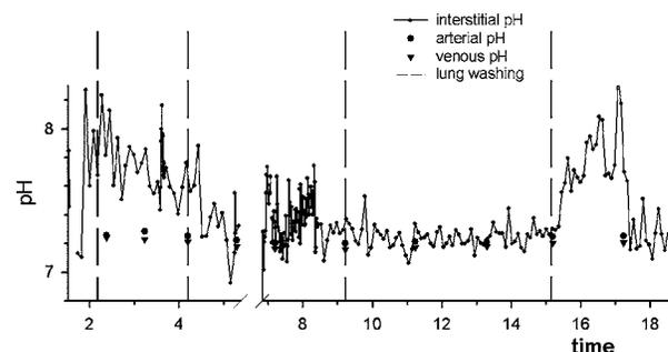
**Fig. 11** *In vivo* measurement on a pig with altered respiratory function. Values of arterial and venous blood measured with a bench-top analyzer are also shown. The dashed lines indicate the times at which the pig was subjected to lung lavages.
