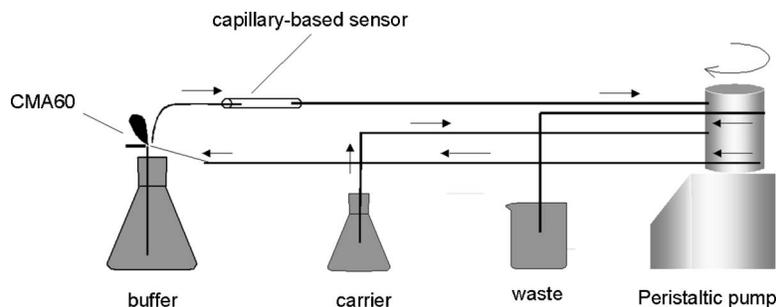
Fig. 3 Setup of the fluidic system for the microdialysis measurements.
