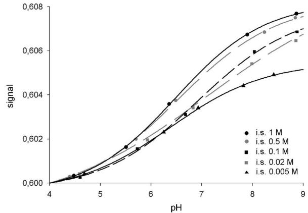
**Fig. 8** Calibration curves at different ionic strength obtained with the Britton-Robinson buffers.
