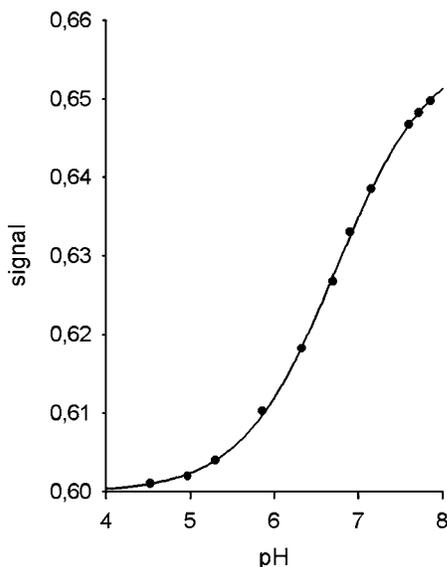
**Fig. 7** Calibration curve of the 10% APTS sensing capillary, the response curve of which is shown in Fig. 6.
