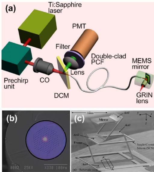
**Fig. 1** (a) The nonlinear optical endoscope system using a double-clad PCF, a 2-D MEMS mirror, and a GRIN lens. (b) Overlay of scanning electron microscopy (SEM) image of a double-clad PCF and the output patterns at wavelengths 410 nm and 800 nm shows the single-mode delivery in the fiber core at a near-infrared wavelength and the multimode propagation of visible light through the inner cladding. (c) SEM image of the MEMS mirror. The entire size is 2.7 mm  $\times$  1.9 mm  $\times$  1.2 mm.
