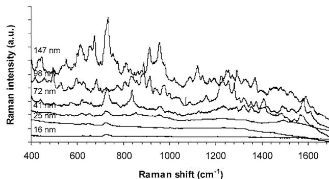
**Fig. 7** Influence of gold nanoparticle size on SERS spectrum of *B. megaterium*.
