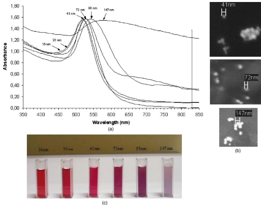
**Fig. 2** (a) UV-visible absorption changes of colloidal gold (16, 25, 41, 72, 98, and 147 nm). (b) SEM images of selected sizes of gold nanoparticles. (c) Color change of gold colloidal suspension as the size changes (color online only).
