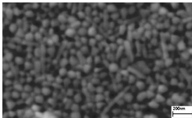
**Fig. 1** SEM image of silver nanoparticles synthesized with citrate reduction method.
