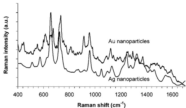
Fig. 5 SERS spectra of *B. megaterium* with gold and silver nanoparticles using a laser at 830-nm wavelength.
