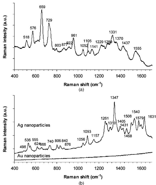
Fig. 4 SERS spectra of *E. coli* with (a) silver nanoparticles at 830-nm wavelength, and (b) gold and silver nanoparticles at 514-nm wavelength.
