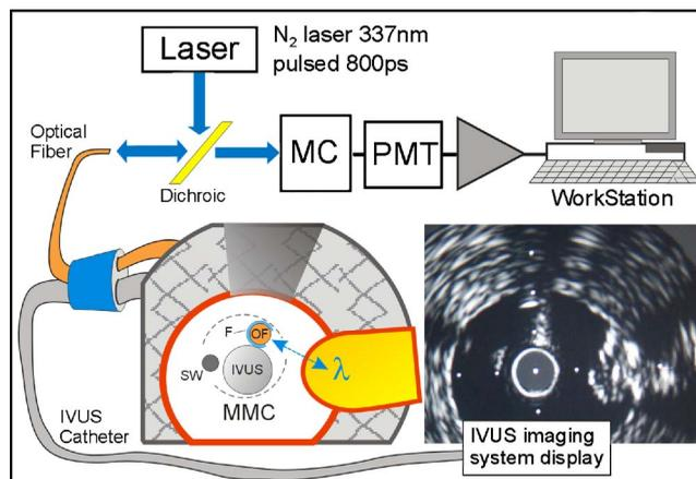
**Fig. 1** A simplified system diagram showing the optical and ultrasound pathways to support the MMC. A cross section of the distal end of the MMC is shown in a phantom artery with a fluorophore target plug placed in the wall. IVUS imaging can clearly orient the SVOF (OF) within the water flushing lumen (F) during the entire positioning procedure.
