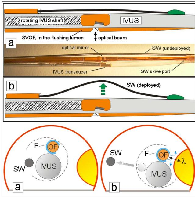
**Fig. 2** Schematic and picture of the three-component construction of the MMC with deployment of lateral (steering) movement with the steering wire (SW). The normally compact MMC components are separated in the photo for clearer viewing. The SW in the undeployed state (a) is near the IVUS sheath and is mounted so that deployment (b) by pushing on the wire will move the MMC close to the fluorophore target in the phantom artery wall.
