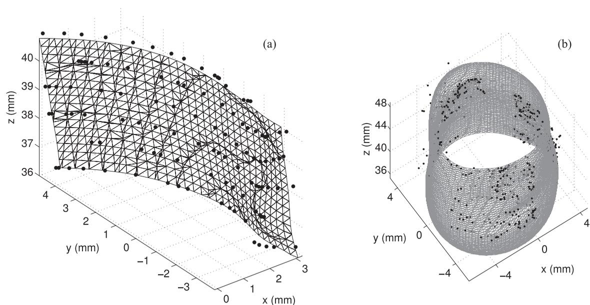
**Fig. 4** (a) Measurement on a metallic cylinder. The configuration using a single fiber with a ball lens to extend the illuminated area was used (see text for detailed optical configuration). (b) Measurement on a paper cylinder, using the setup shown in Fig. 1, with three fibers for illumination.
