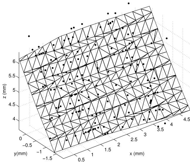
**Fig. 3** Validation measurement on a tilted plane. Representation of the measured points (black dots) along with the interpolating surface (mesh).
