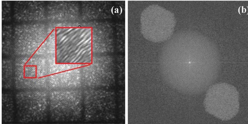
**Fig. 2** (a) Typical signal when observing a perpendicular plane made of white paper containing a 2-mm grid. (b) Fourier spectrum of (a).
