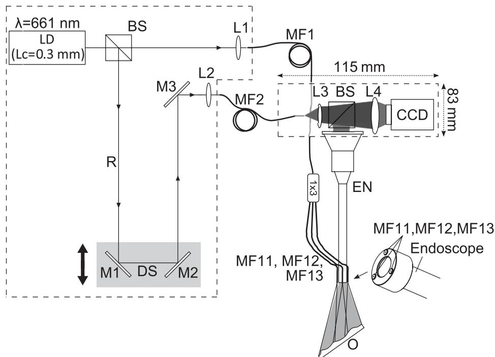
**Fig. 1** Schematic of the setup. LD: laser diode. BS: beamsplitter. M1, M2, and M3: mirrors mounted on a motorized translation stage. L1 through L4: lenses. CCD: charged-coupled device camera. EN: rigid endoscope (Karl Storz 10320A). MF: monomode fibers. R: reference wave. O: object.
