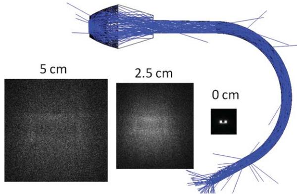
**Fig. 4** Optical simulation of light pipe efficiency showing light distribution for several distances from the tip.
