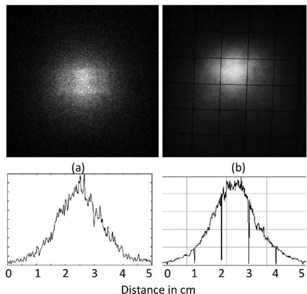
**Fig. 6** (a) Simulated and (b) measured light distribution over a  $5 \times 5$ -cm area at 1-cm distance.
