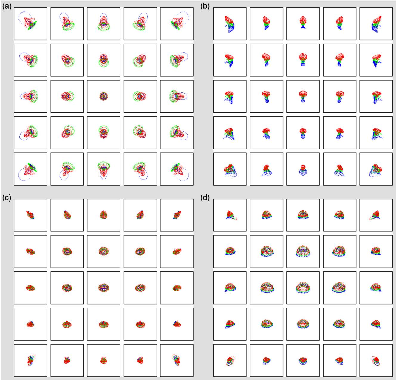
**Fig. 3** Spot diagram for on-focus cases for (a) ch. 1, (b) ch. 2, (c) ch. 3, and (d) ch. 4. The  $5 \times 5$  cells represent the FOV of  $1 \text{ k} \times 1 \text{ k}$  CCD. The size of each cell corresponds to 1 arc sec. Colors indicate simulated images of the shortest (blue), mid (green), and longest (red) wavelength in each channel. Specifically, 400, 470, 550 nm for ch. 1, 550, 630, 700 nm for ch. 2, 700, 760, 820 nm for ch. 3, and 700, 800, 950 nm for ch. 4.
