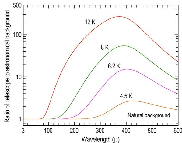
**Fig. 2** A comparison of telescope emission (effective emissivity = 0.05) compared to the sky background in the mid to far infrared.
