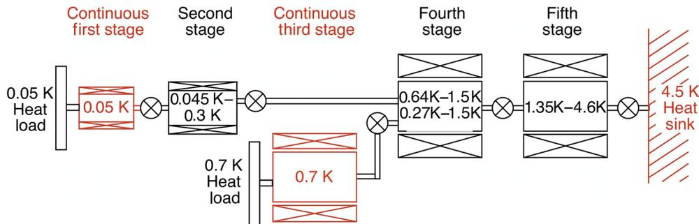
**Fig. 6** A schematic representation of the FIP and OSS CADR. The ADR stages are synchronized to move heat from the 50-mK and 0.6 K stages to the 4.5 K stage, where it is lifted by the 4.5 K cryocooler(s). Salt pill operating temperature range is indicated. The average cooling power for each continuous stage and heat rejection to the sink are indicated in red as they are called out in instrument requirements.
