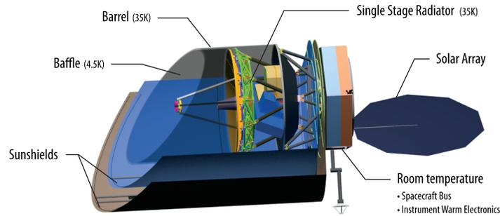
**Fig. 1** Origins temperature zones are designed to maximize cryocooling efficiency while ensuring a 4.5 K environment for the telescope and instruments. The instruments are housed in the 4.5 K zone beneath the primary mirror.
