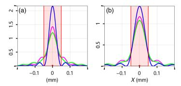
**Fig. 6** The one-dimensional PSFs on the slit plane at (a) 9.98108  $\mu$ m and at (b) 15.23428  $\mu$ m of the wavelength. The vertical axis is the relative intensity. The blue, magenta, and green curves indicate the cases of aberration-free, astigmatism, and spherical aberration, respectively. The red filled area indicates the width of the slit aperture.
