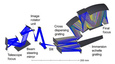
**Fig. 2** The optical design of the SPICA/SMI-HR. The rays are colored by the diffraction orders of the diffraction by the immersion echelle grating. The HR spectrometer is one of four subunits that compose the SPICA/SMI.<sup>15</sup>
