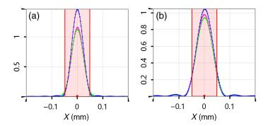
**Fig. 7** The one-dimensional PSFs on the final focal plane at (a)  $9.98108\mu m$  and at (b)  $15.23428\,\mu m$  of the wavelength. The vertical axis is the relative intensity. The blue, magenta, and green curves indicate the cases of aberration-free, astigmatism, and spherical aberration, respectively. The red filled area indicates the width of the slit aperture.
