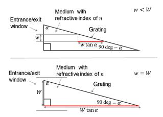
**Fig. 1** Illustration of the calculation of the round-trip optical-path difference between light rays from the opposite ends of the beam on the incident (exit) window. The upper panel is for the case w < W, and the lower panel is for w = W. The lengths of the solid red lines show half of the round-trip path difference between light rays from the opposite ends of the beam on the incident (exit) window.
