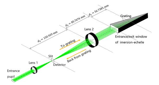
**Fig. 3** Optical layout model used for the simulations. The thicknesses of the lenses are exaggerated in this figure to make them easy to see. In the actual simulations, we used spatial phase modulations to represent thin lenses with zero thickness. The surface-to-surface distances  $d_1$ ,  $d_2$ , and  $d_3$  shown here have the same definition used in Appendix B; see also Table 1.
