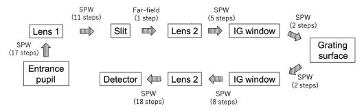
**Fig. 4** Summary illustration of the method of calculation. The abbreviation SPW represents a method that uses a spectrum of plane waves, and IG is an abbreviation for immersion-echelle grating. We need the division of the propagation distances to reduce the amount of random-access memory that SPW requires. However, for the slit-less cases, we calculated the propagation between lenses 1 and 2 using SPW (1 step), which is different from this figure.
