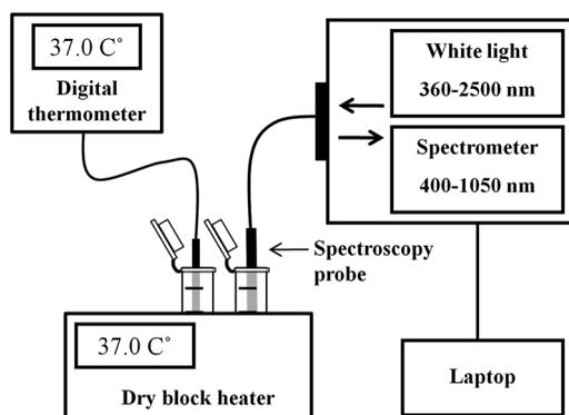
Fig. 1 Schematic overview of the spectroscopy setup.
